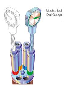
For the manual measurement of the multipoint Extensometers, a dial gauge, a digital caliper or the portable electronic displacement transducer with digital readout unit is used.
