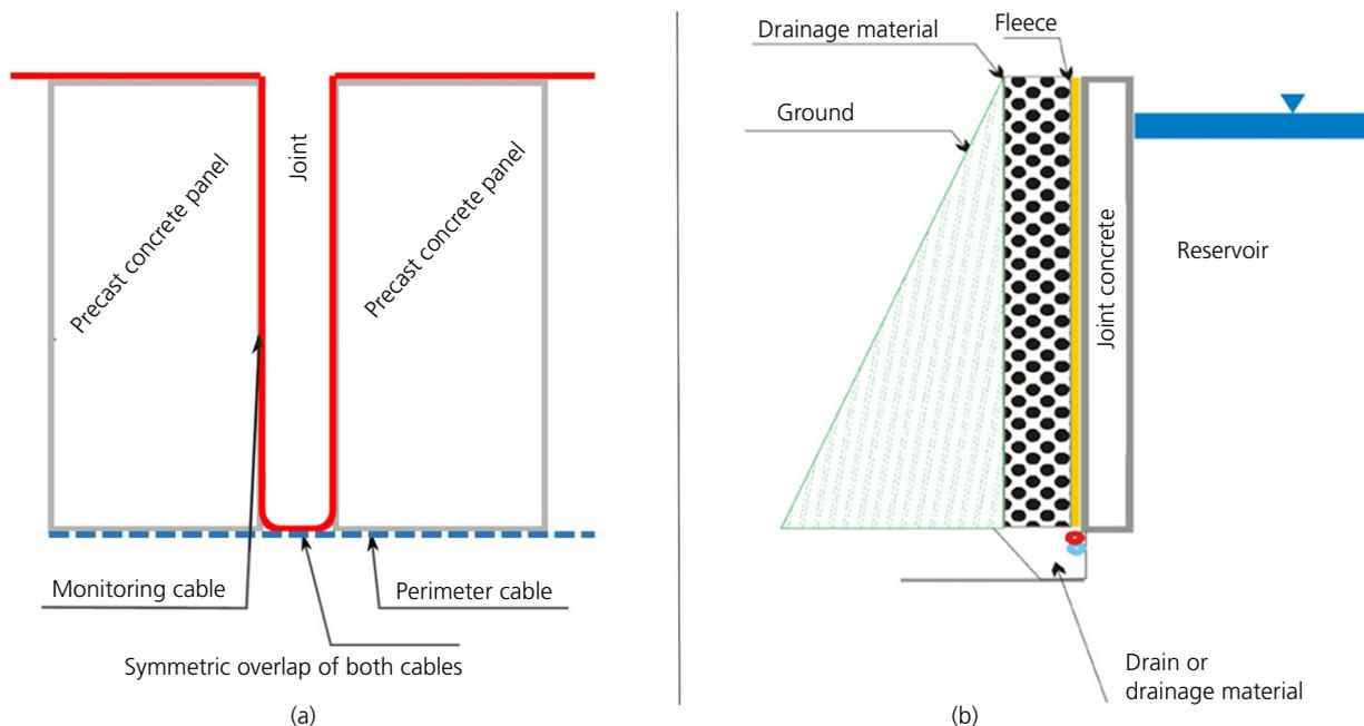
**Figure 3.** Location of cable placement at the external walls with the monitoring cable: (a) elevation view; (b) cross-section
