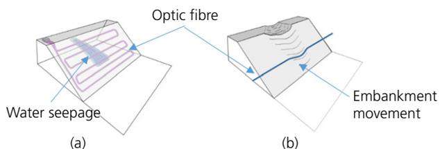
**Figure 1.** Basic principle of fibre optic sensing for leakage (a) temperature and movement (b) strain) monitoring in embankments
