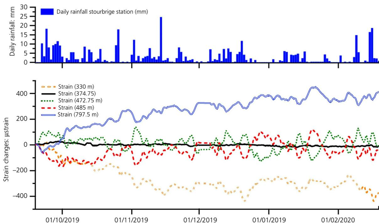
Figure 8. Strain variation at five selected locations along loop 2, and comparison with rainfall data. Location given in Figure 9
