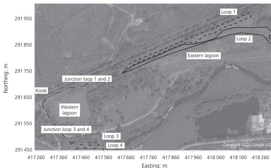
Figure 6. Curdworth sludge lagoon: site description and fibre optic cable layout
