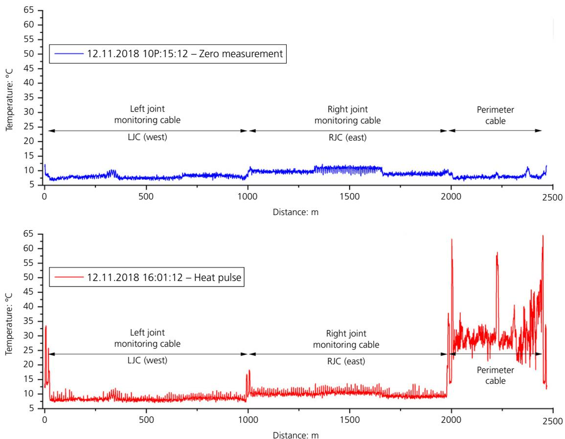
Figure 4. Temperature spikes (0–2000 m) caused by the heat-pulse measurement of the perimeter cable were used for the calibration of the position of the monitoring cable
