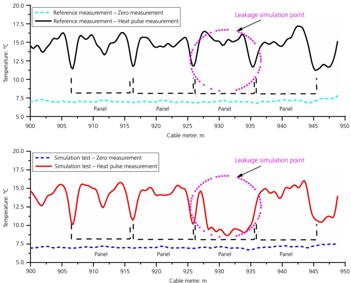
**Figure 5.** Comparison of the heat pulse of the reference measurement and the simulation test. A significant lower temperature change can be observed for the cable metres 926–936 m
