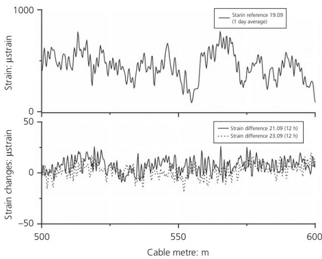
Figure 7. Strain absolute values and strain changes for one 100 m long section of loop 1 on 19 September 2019
