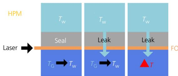
**Figure 2.** Detection of a leak with an optical fibre (FO) installed behind a thin sealing layer. To the left, a no-leak situation, where the water temperature  $T_w$  equals the ground temperature  $T_g$  along the optical fibre FO. In the centre, a leaking situation, with  $T_w$  equals  $T_g$ . To the right, necessity to create an increase of temperature  $\Delta T$  by using the heat-pulse method
