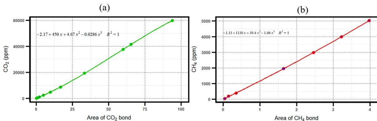
**Figure 4.** The calibration curve of CO<sub>2</sub> (a) shows a polynomial fitting of the CO<sub>2</sub> calibration curve on FTIR ranging from 101 ppm to 59,806 ppm. As for the CH<sub>4</sub> (b), the highest concentration that was applied was 5000 ± 99 ppm, with an average absorbance area (Abs) of 3.97 ± 0.012. The lowest concentration tested was 50 ppm, with an average absorbance area of 0.046 ± 0.024 (resolution: 1 cm<sup>-1</sup>).
