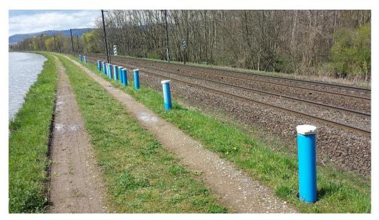
Automatic Leakage Detection System of temperature anomalies. Flow velocities are calculated automatically and alarms are automatically send by flow velocities >  $10^{-3}$  m/s. The data loggers (protected in blue tubes) are connected to the measuring chains and send the measuring data via modem for further automated processing.
