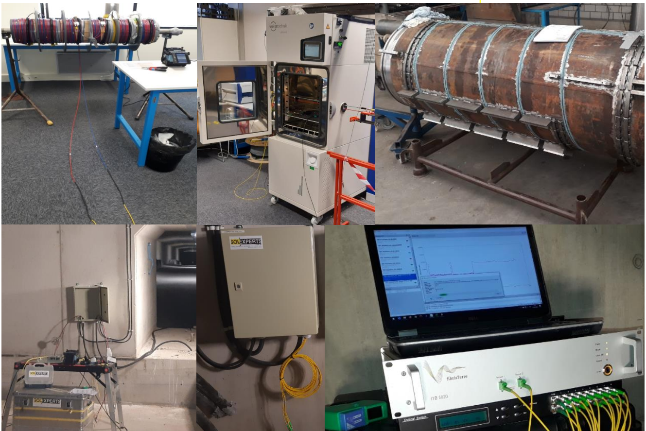
Preparation/calibration of the cables in the workshop, installation on the structure, connection to the interrogator
