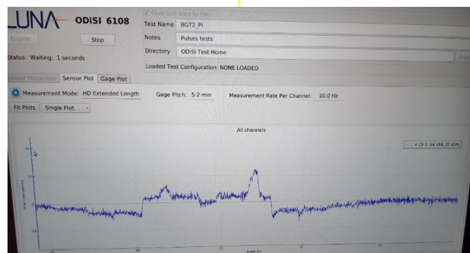
LUNA ODiSI-6108 Rayleigh OFDR Interrogator / Measurements with high frequency and high spatial resolution
