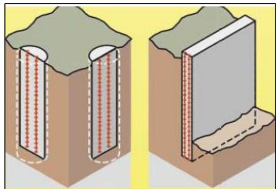
**Figure 2.13 shows the use of sliding micrometer at piles and diaphragm walls.**
