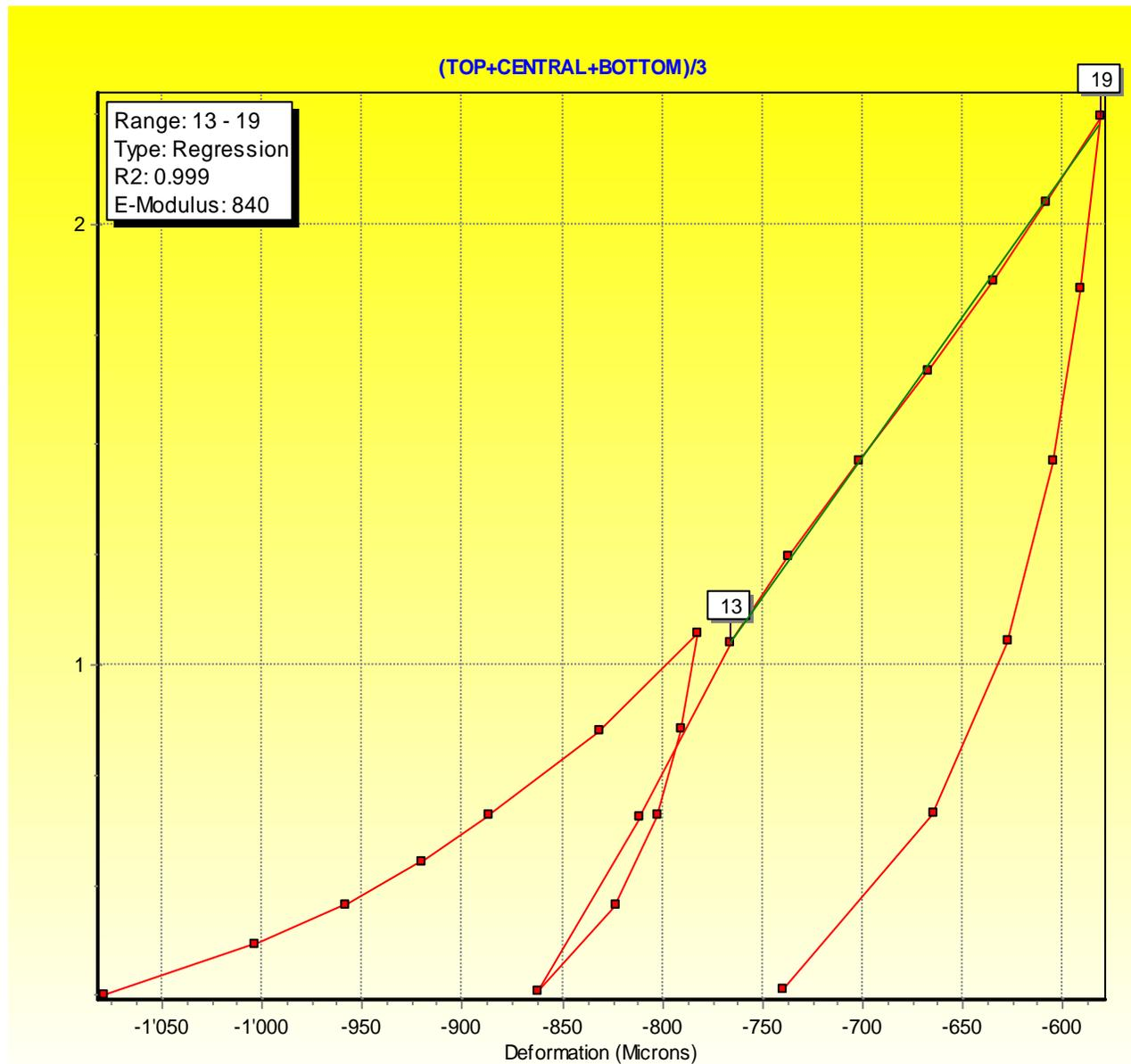
A measurement of 0 micron corresponds to the reference tube diameter (100 mm)
