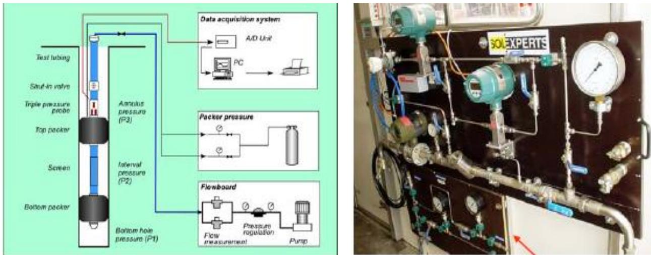
**Figure 3.5 shows double packer test equipment arrangement for testing after borehole is completed.**
