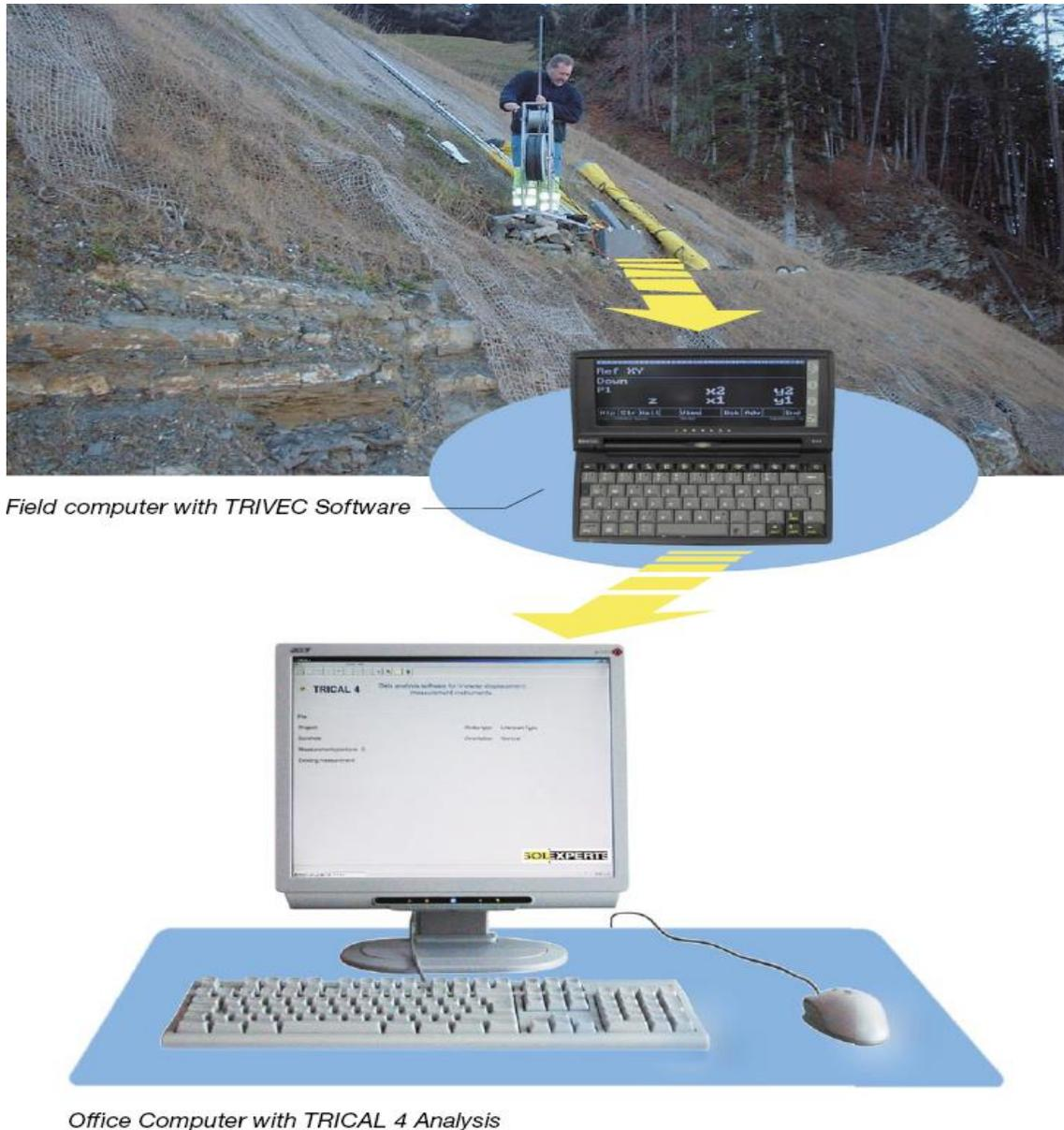
**Figure 4.1 shows the monitoring system how the data is received directly to the office computer and analysis by another program TRICAL4.**
