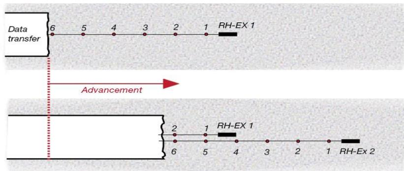
**Figure 2.18 shows the application of the Reverse Head Extensometer in Alptransit Gotthard tunnel Switzerland.**
