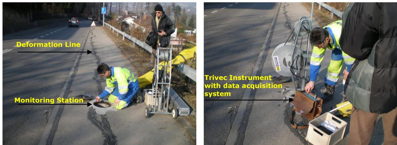
**Figure 6.14 shows the measurement of slope movement  $X$ ,  $Y$  and  $Z$  vector by Trivec probe on road side slope at Maur.**
