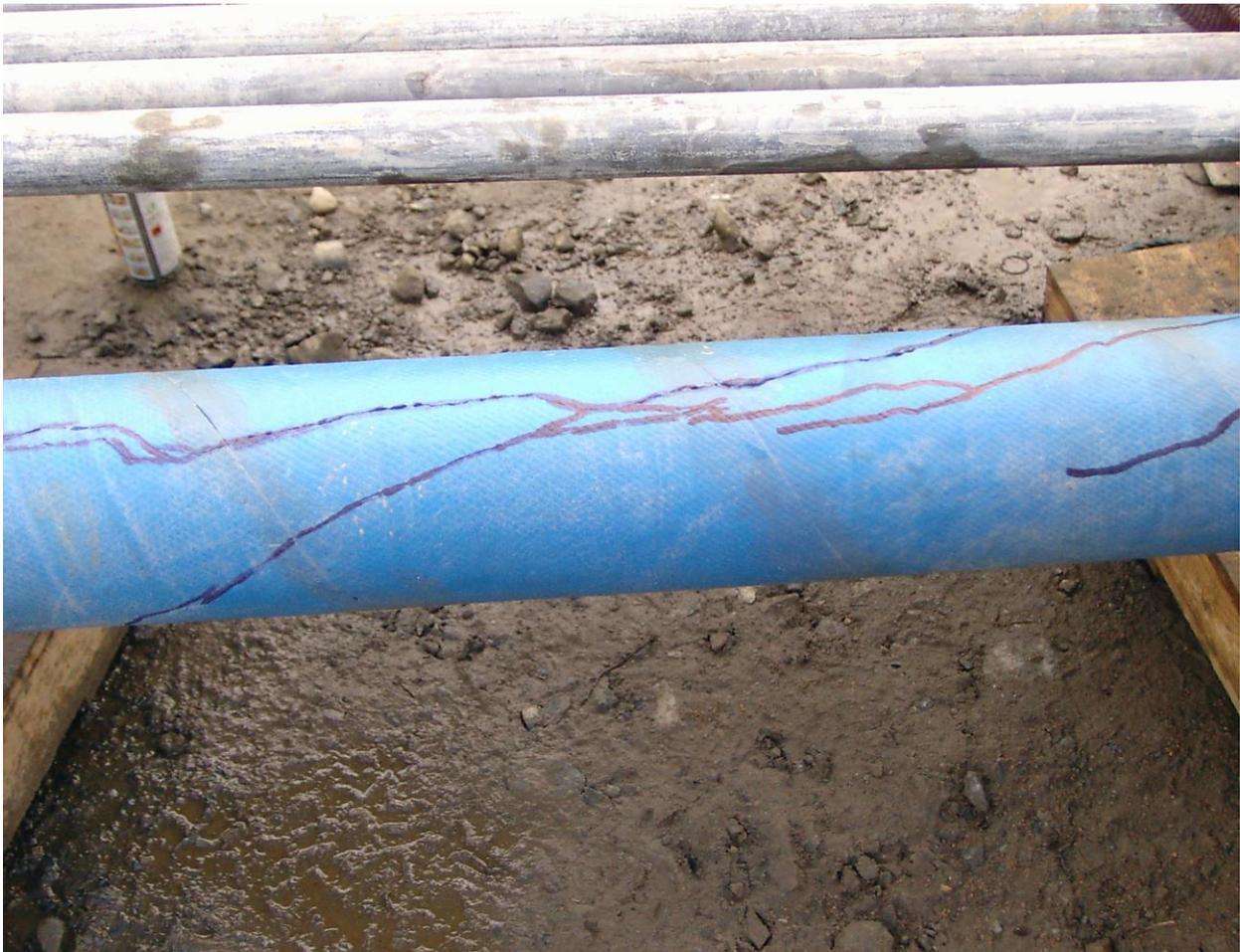
***Figure 2.47 Impression packer of hydrofracture test with traces of included features.***
