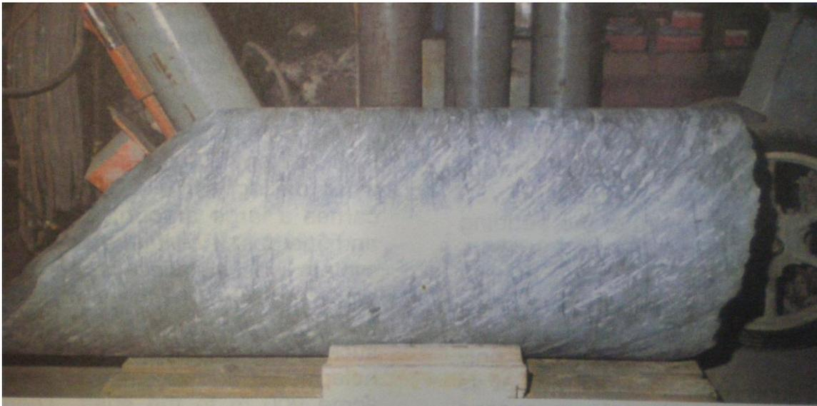
**Figure 6.10 Shown a 2.5 m long 600mm diameter double core barrel sample.**
