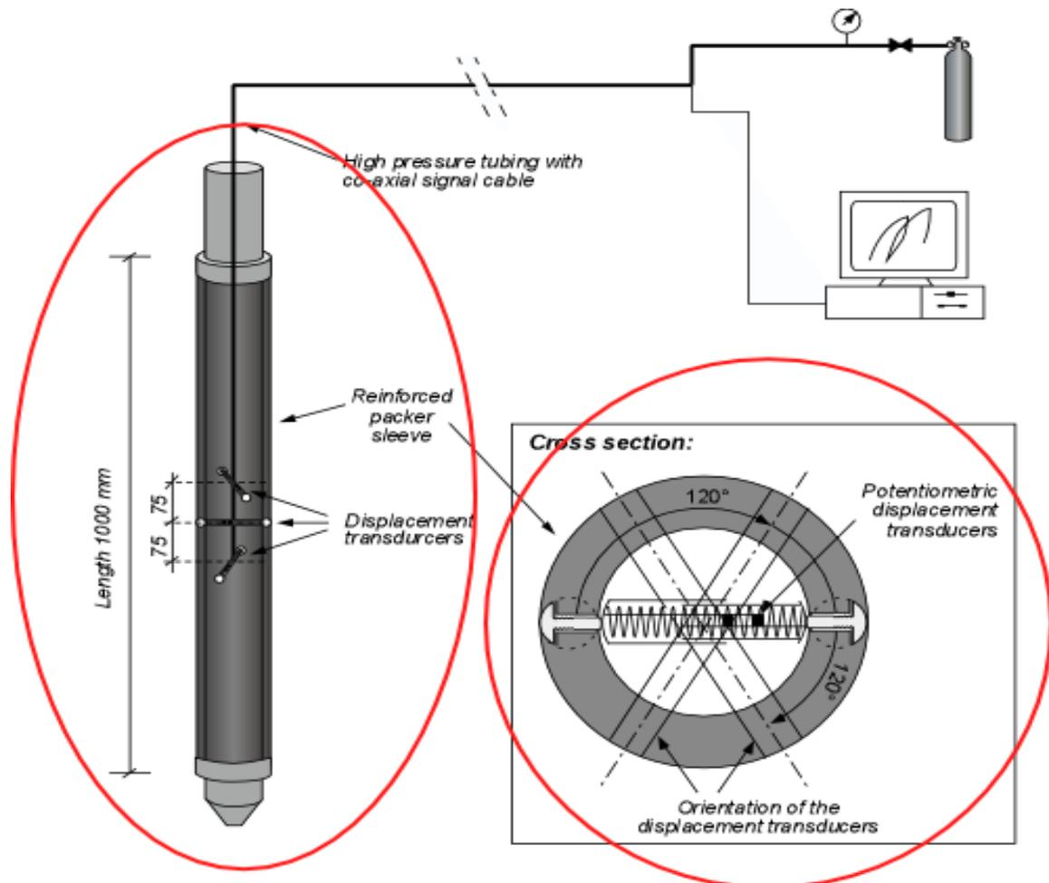
Figure 2.34 shows the internal structural details of the dilatometer probe
