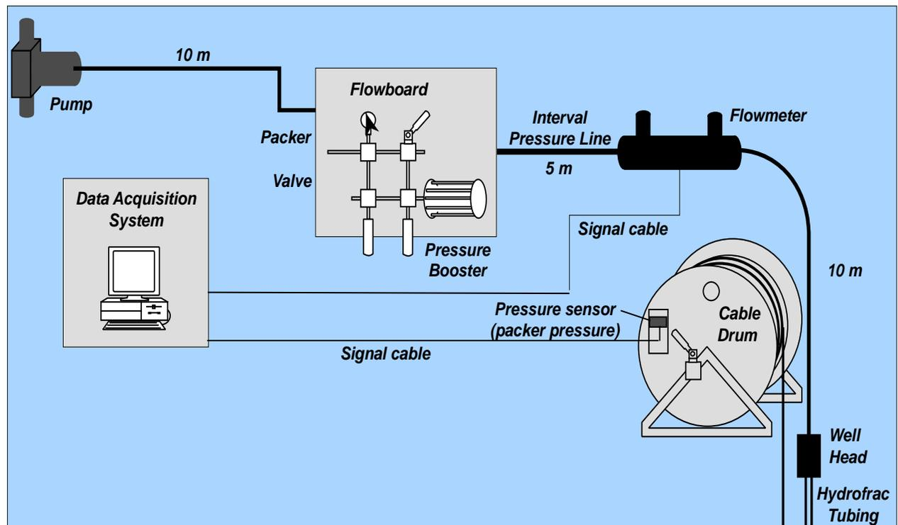
Figure 2.45 showing the arrangement of the surface equipment arrangement.
