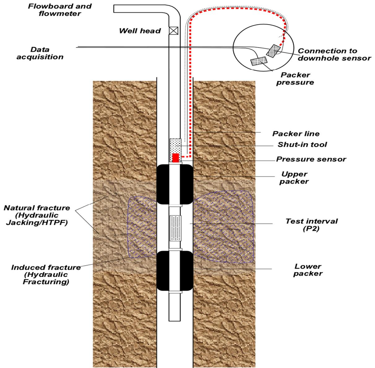
**Figure 2.44 showing the arrangement of the borehole equipments and testing procedure.**
