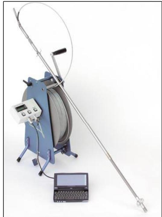
*Figure 2.5 shows a complete set of sliding deformer.*
