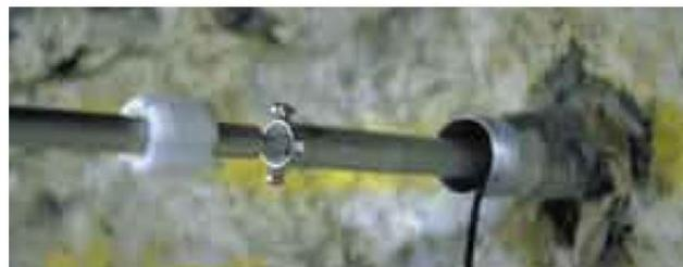
**Figure 2.21 shows the application and installation of Fixed Re-Installable Micrometers in a borehole.**
