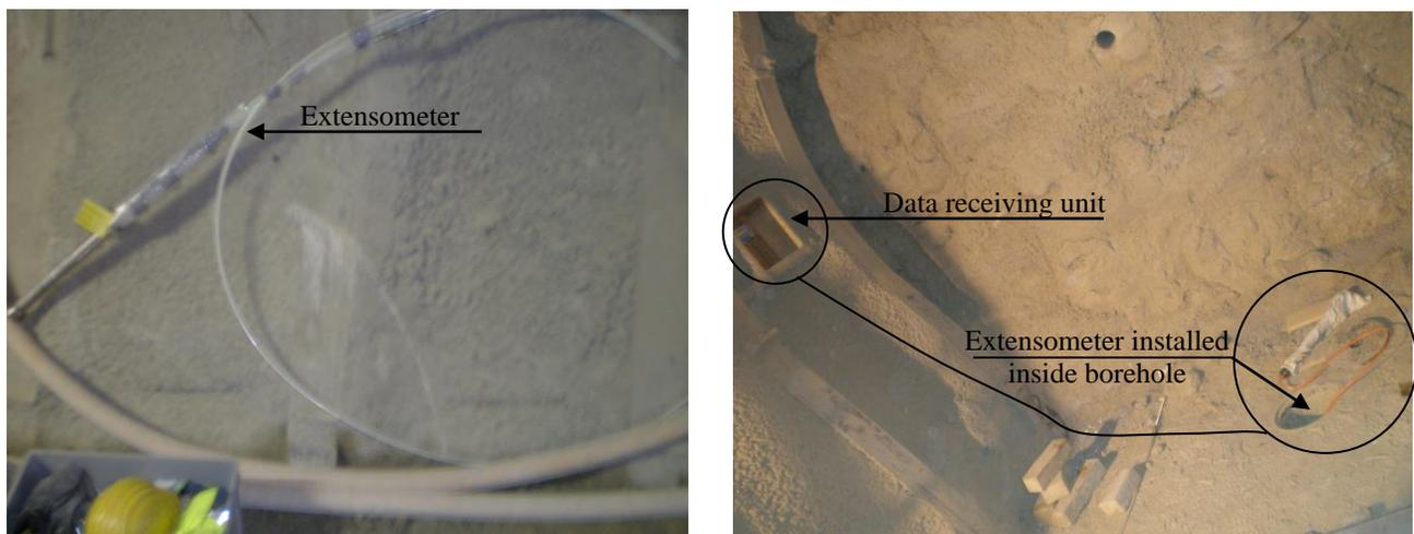
**Figure 6.6 a and b shows the installation of the extensometer in the borehole.**
