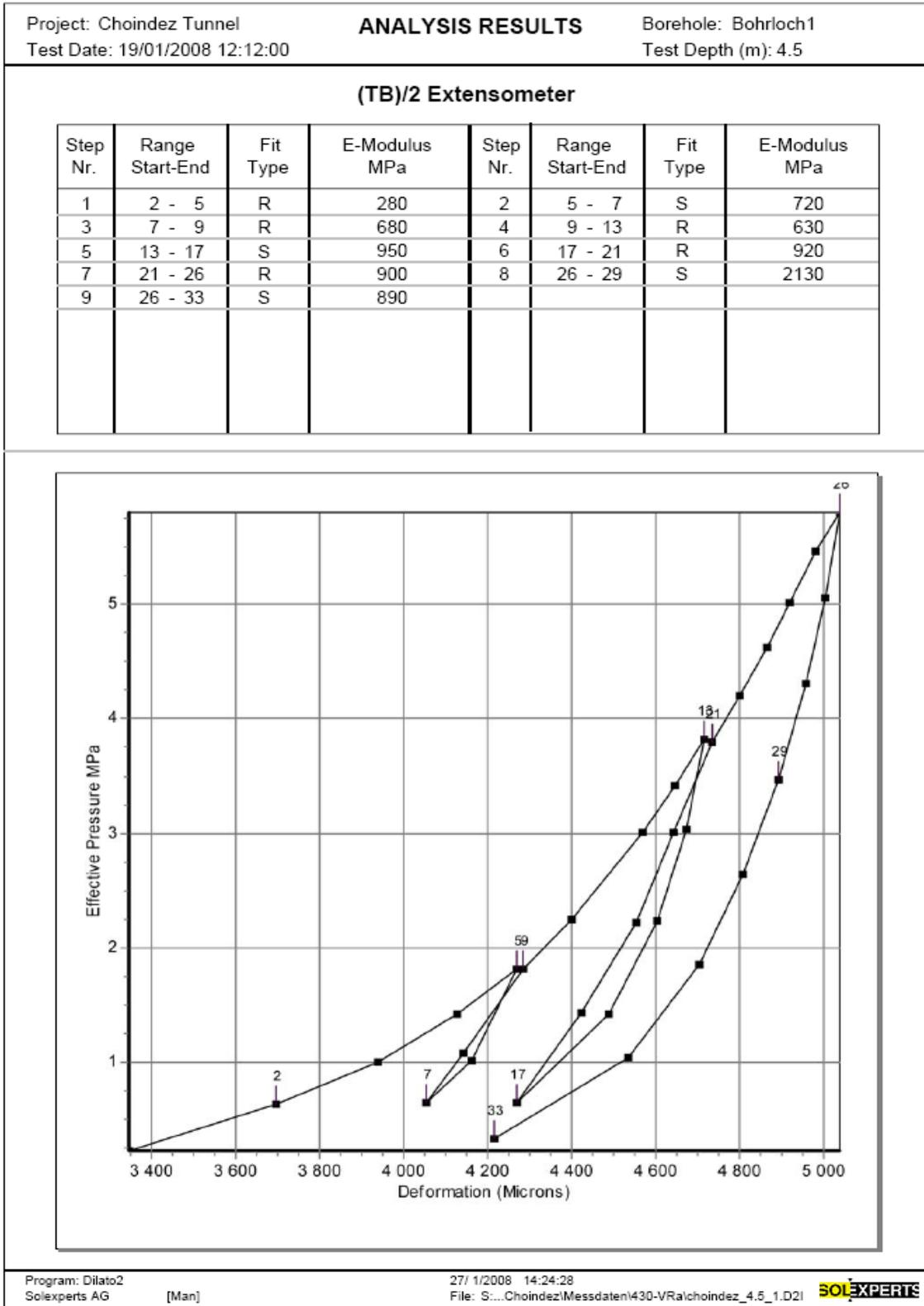
**The above presented chart and data is an example of the dilatometer test result at the depth of 4.5m.**
