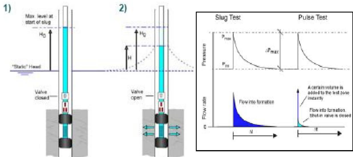
**Figure 3.8 represents the principle of Slug test and Slug/pulse test.**
