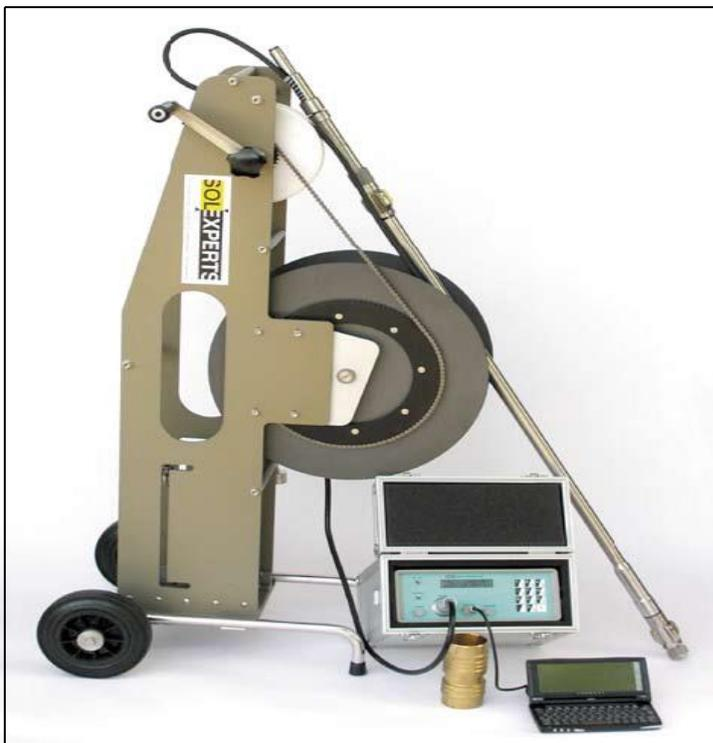
**Figure 2.10 shows complete set of Sliding micrometer and internal details of the probe.**
