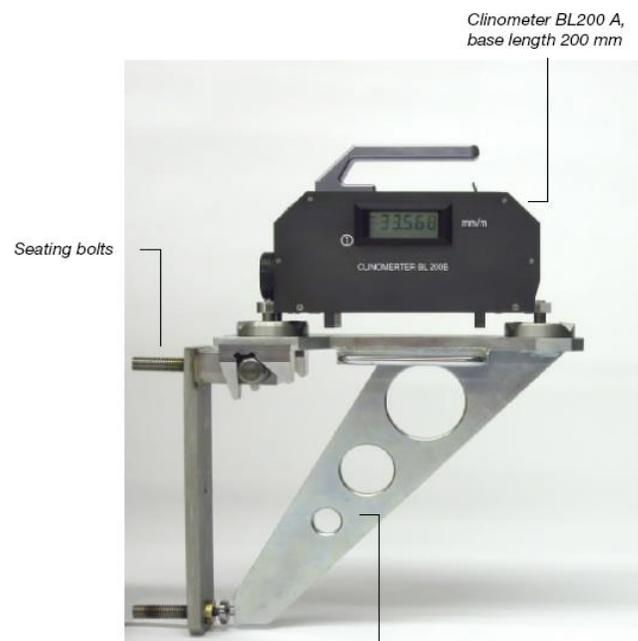
Figure 2.28 shows the instrument set up and use Clinimeter BL200B.
