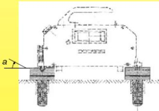
Clinometer calibration device KMK-1000 for periodic control of sensitivity, linearity and zero drift of the instrument
