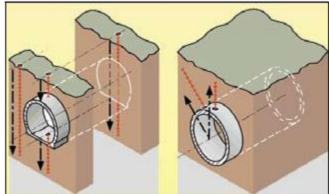
**Figure 2.12 shows the application of sliding micrometer in tunnels**
