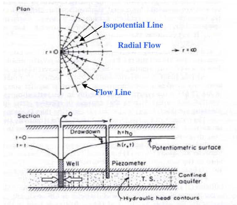
Figure 3.1 shows single well, interference test (Cross hole test).
