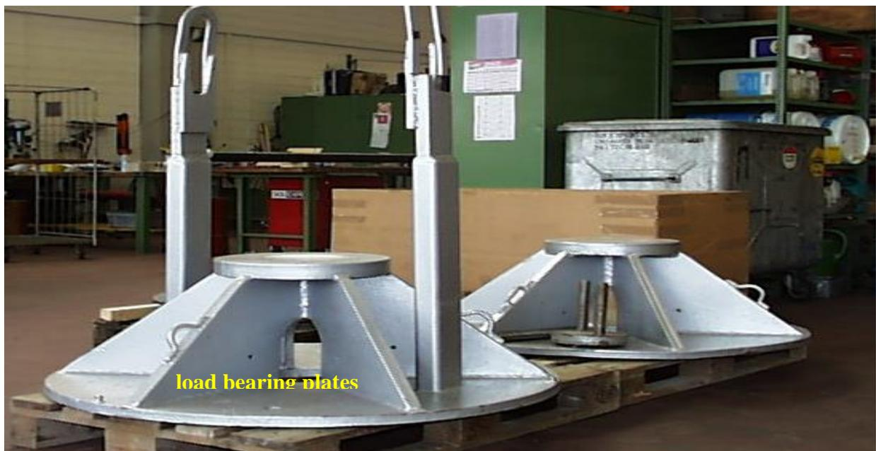
**Figure 2.40** shown the loading plates prepared at workshop for the plate loading test.
