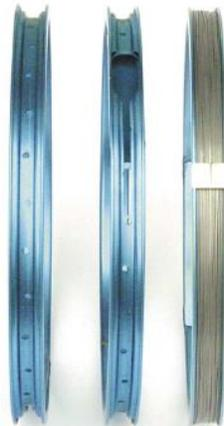
The individual Invar wires of successive lengths are stored on spools in a storage case
