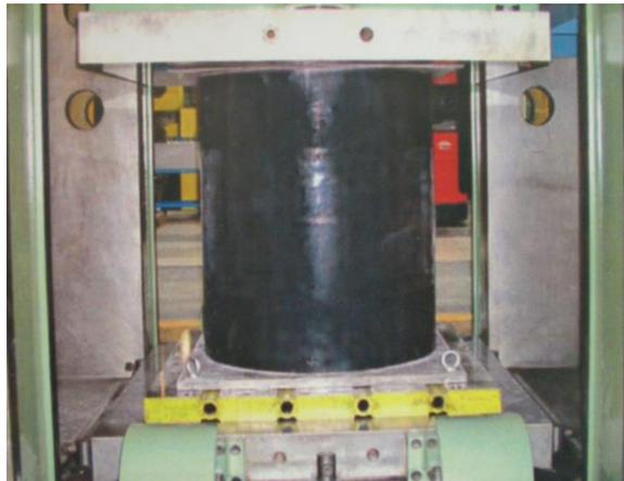
a) Load test of hiDCon foundation elements in protection sleeve  $\phi=900$  mm, and  $H=1000$  mm
