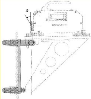
Seating bolts VB, for measuring change in inclination in the vertical plane parallel to the wall.
