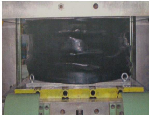
c) Load test of hiDCon foundation elements
