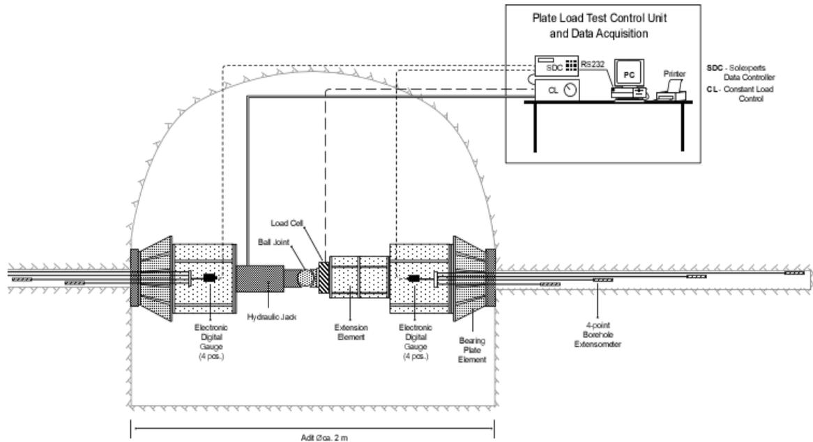
**Figure 2.39** an sketch of the complete setup of the plate loading test.
