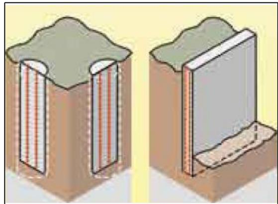
*Figure 2.2 shows the positioning and use of Trivec on pile for three dimensional (X-Y-Z) deformation measurements.*
