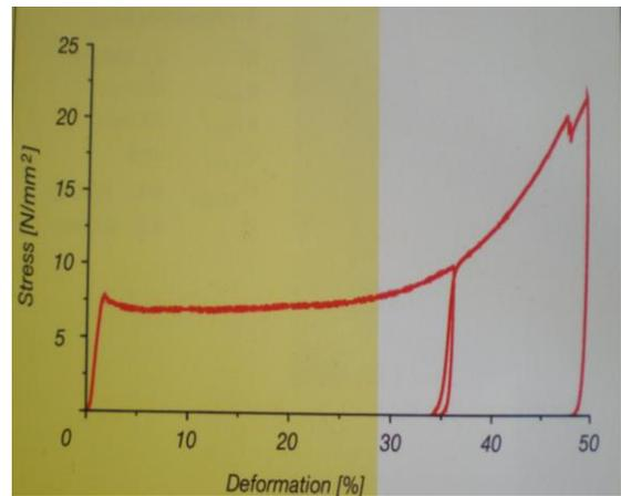
d) Stress strain diagram of a hiDCon foundation element
