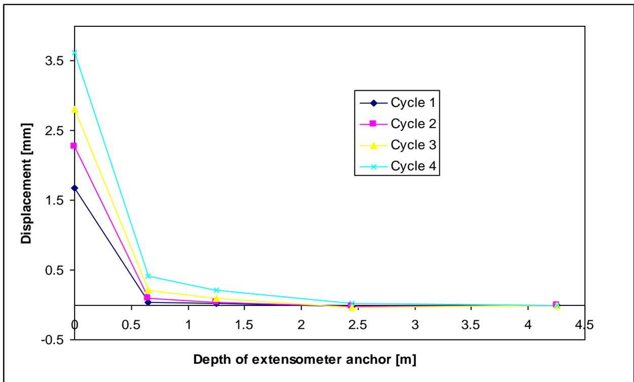
Figure 2.42 shows results of displacement measurements at the surface of the loading plate (depth=0m) and with four extensimeter underneath the loading plate (depth of anchor: 0.65m, 1.25m, 2.45m and 4.25m).
