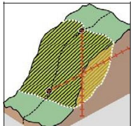
*Figure 2.6 shows the use of sliding deformer at landslide slope.*
