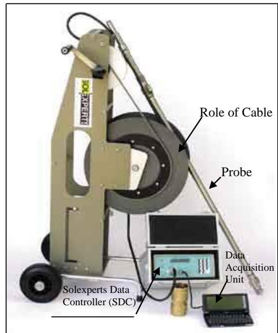
**Figure 2.1 TRIVEC measuring equipment.**
