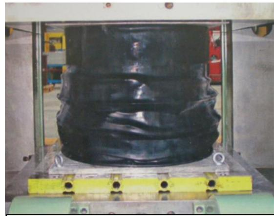
b) Load test of hiDCon foundation elements
