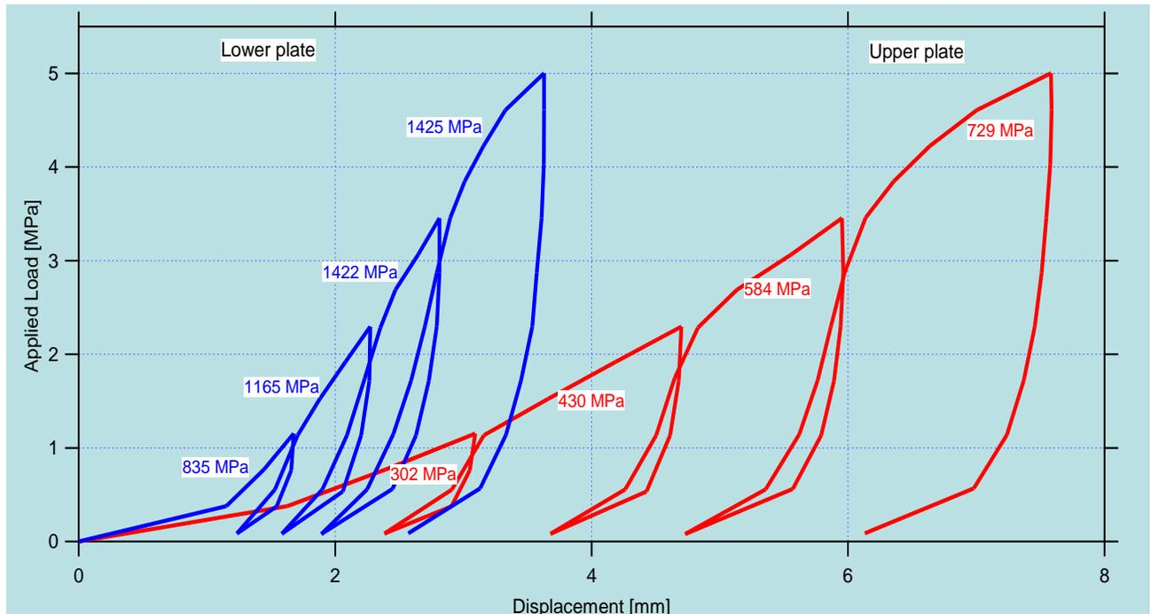
Figure 2.41 an example of plate loading test results with four cycles and corresponding value of the deformation module. A stiffening of the rock mass with increasing rock load is observed with both plates.
