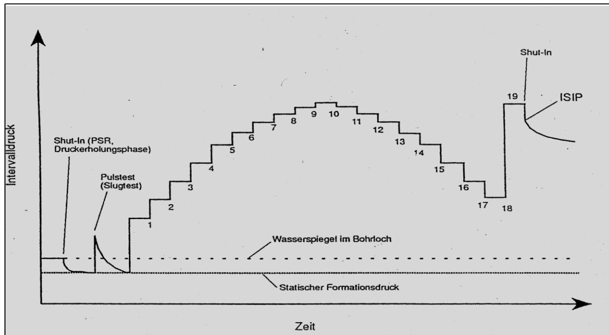
**Figure 2.48 shows a typical hydrojacking test (pressure curve of stepwise injection).**
