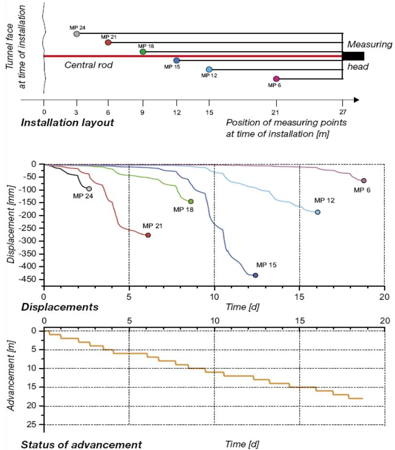
Figure 2.19 shows the application of the Reverse Head Extensometer at Alptransit Gotthard base tunnel Switzerland.
