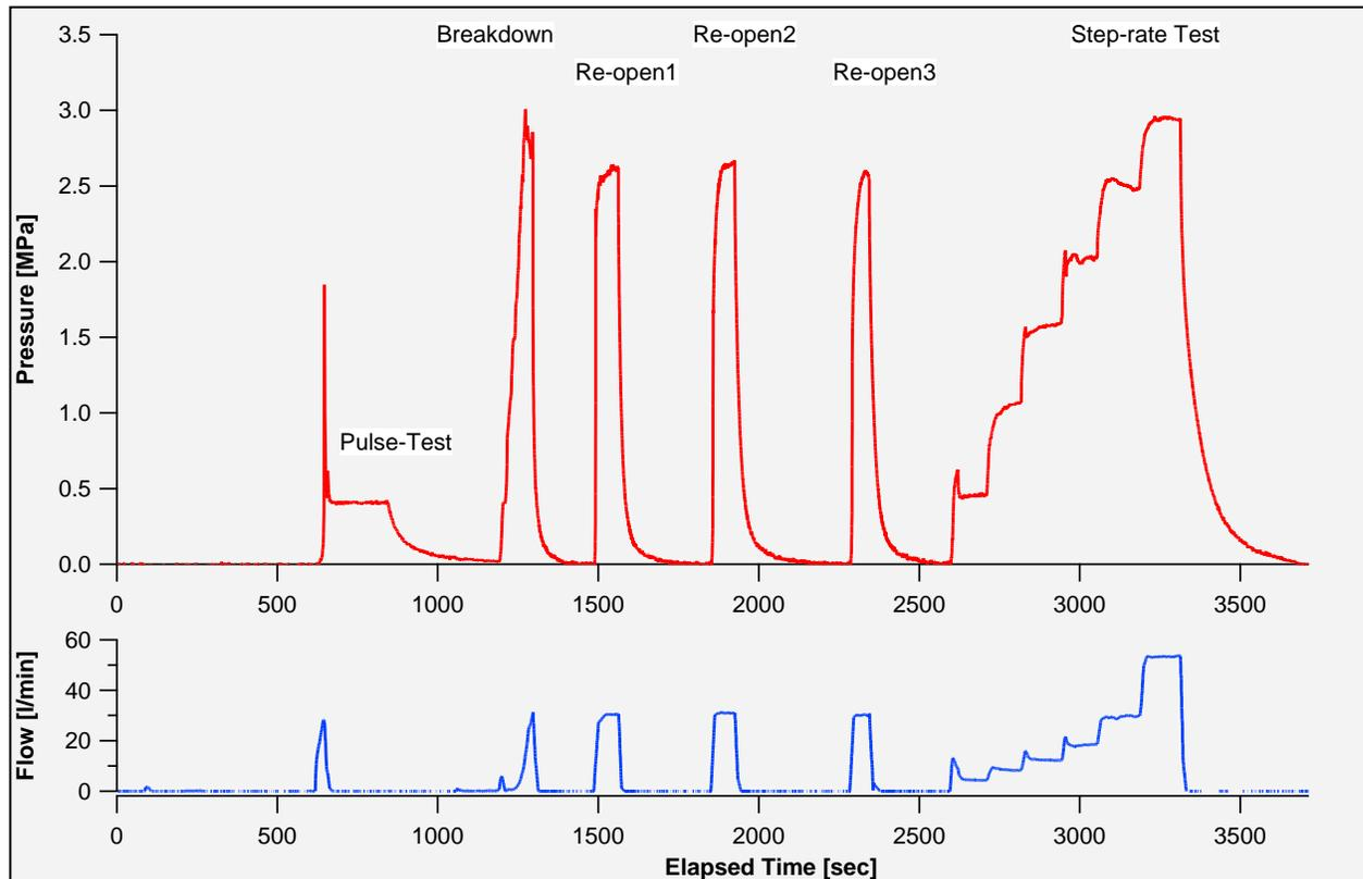
**Figure 2.46 shows the results of hydraulic-fracturing test with breakdown cycle, the re-open cycles and a step-rate test.**
