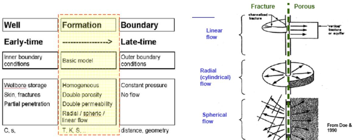
Figure 3.7 shows the flow regimes and flow model in Double Packer test.
