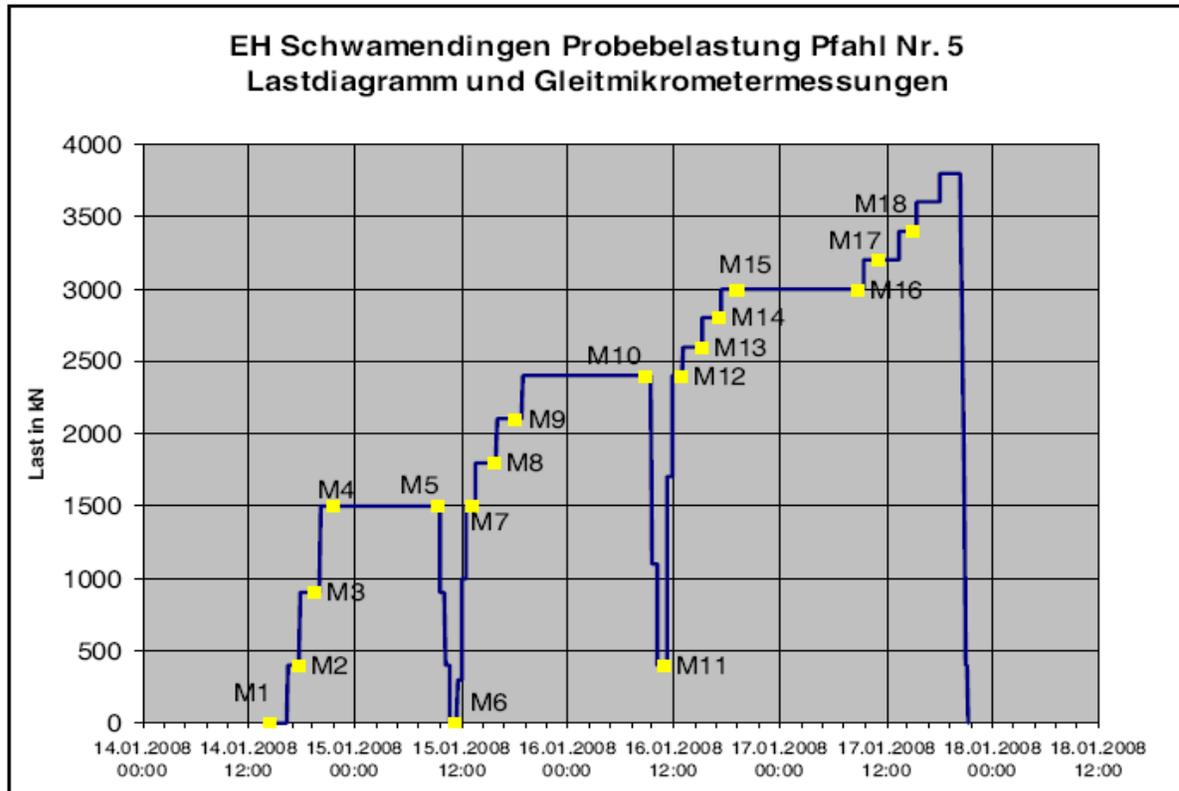
**Figure 6.4 shown test results sliding micrometer, axial deformation during load test.**
