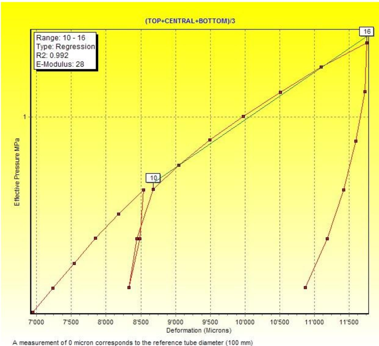
Figure 2.36 shows an example of the test result on soil.
