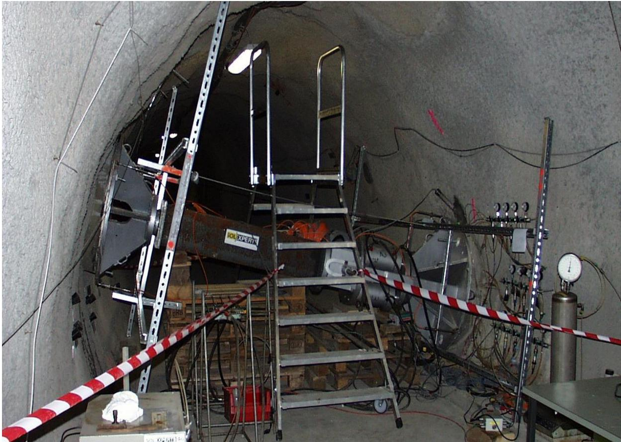
***Figure 2.38 shows the final arrangement of Plate Loading test at Mont Terri Research Rock Laboratory site.***
