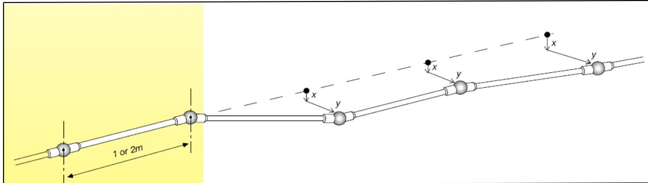
Figure 2.32 shows the function of chain deflectometer in a multiple automatic monitoring of subsurface deformation.
