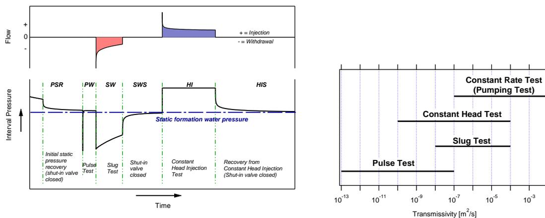
**Figure 4:** left side: Idealised test sequence showing a combination of various hydraulic testing methods.
