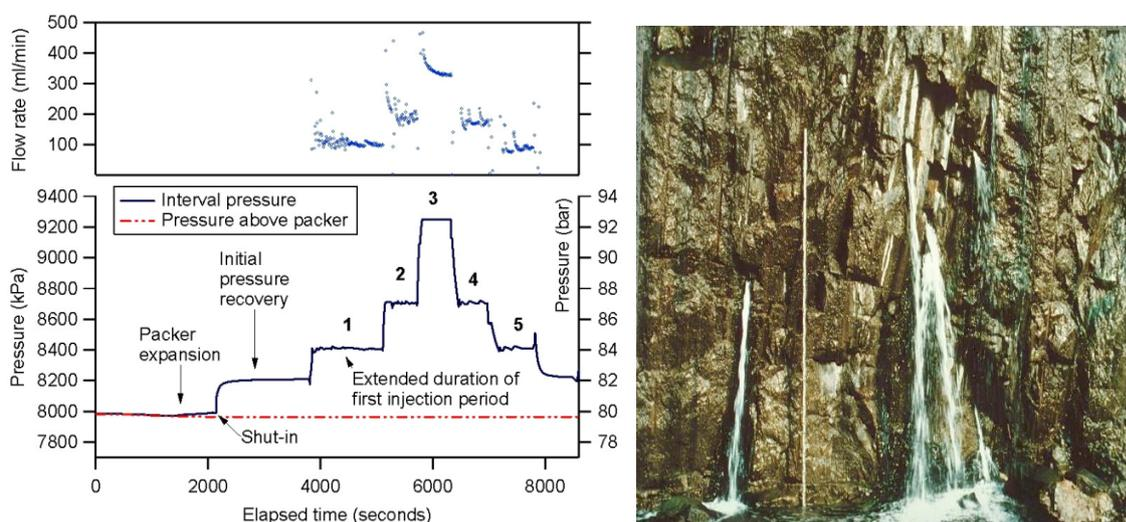
**Figure 3:** left side: Example of an enhanced Lugeon test extracted from the ISO/DIS norm 22282-3 (2006). The initial pressure recovery is usually referred to as PSR (pressure shut-in recovery).
