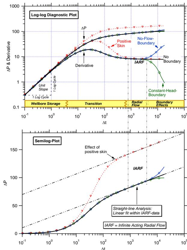
**Figure 5:** upper diagram: log-log plot showing the different flow phases.
