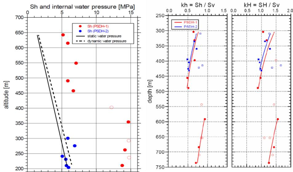
**Figure 1:** Left side: Minimum principle stresses and internal water pressure water pressure vs. elevation.
