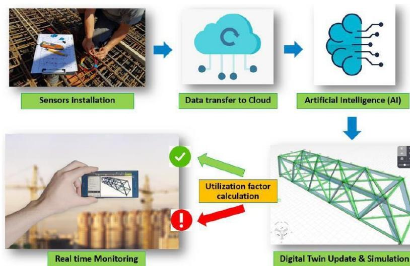
*Figure 2: Operation of the monitoring and predictive analysis system based on digital twin development and calibration, automatic simulation and 3D visualization in the cloud.*
