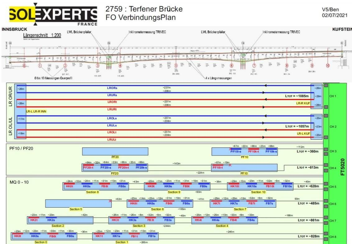
Figure 6: Installation plan of the fiber optic sensors
