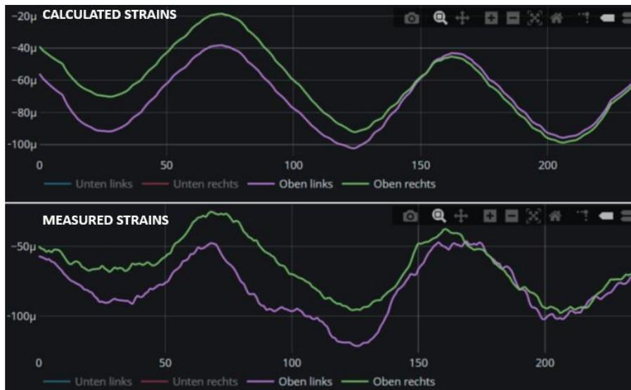
Figure 8: Comparison of calculated and measured strains: the difference is less than 5%.
