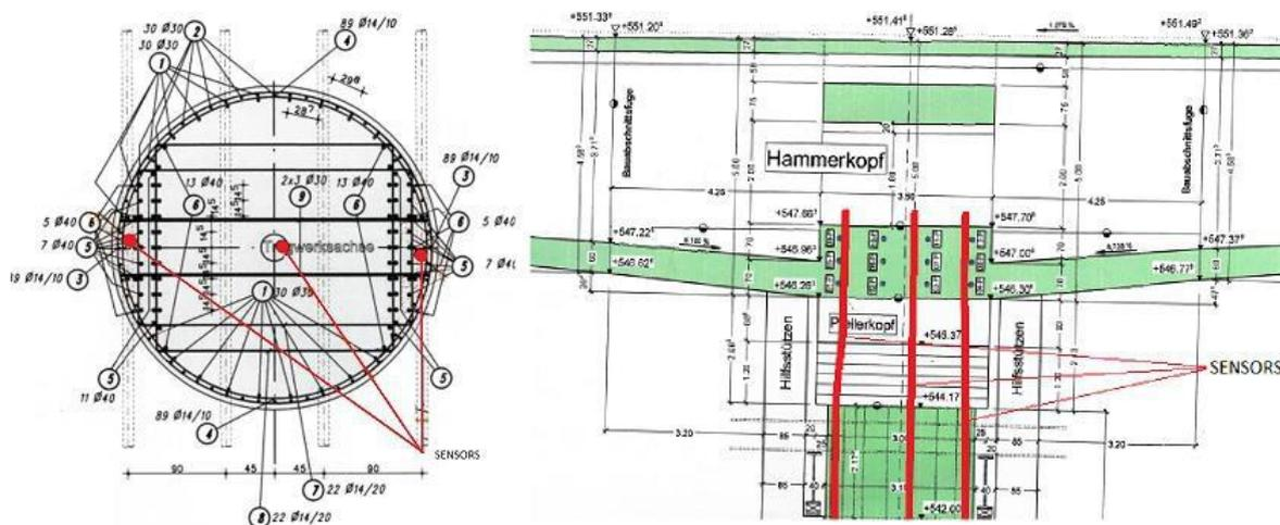
Figure 6: Detail about the sensors installed on the pillars and piles.
