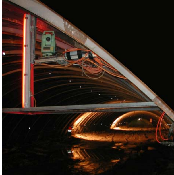
Figure 2.2. Robotic Total Station installed in the tunnel
