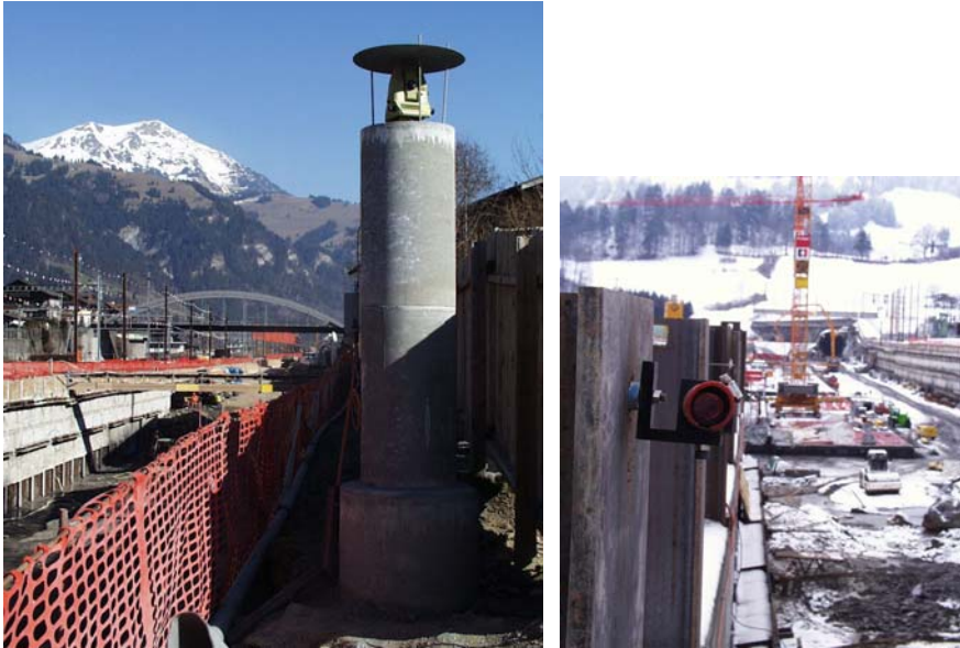
Figure 3.2: Tachymeter Station T1 with measuring point (mini-prism)
