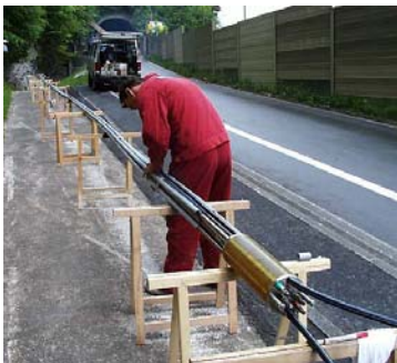
Figure 4.4 Modular Extensometer before installation Figure 4.5 Installed Modular Extensometer
