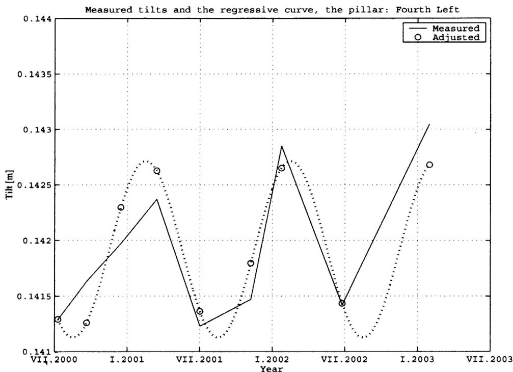
Figure 4: Horizontal shifts of pillar in section 4 left
