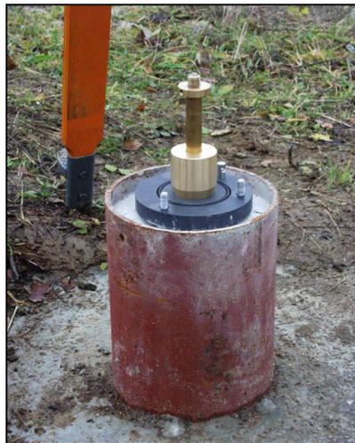
Figure 7: Reference point with insert tool in combined casing and tripod of Leica TC 1800
