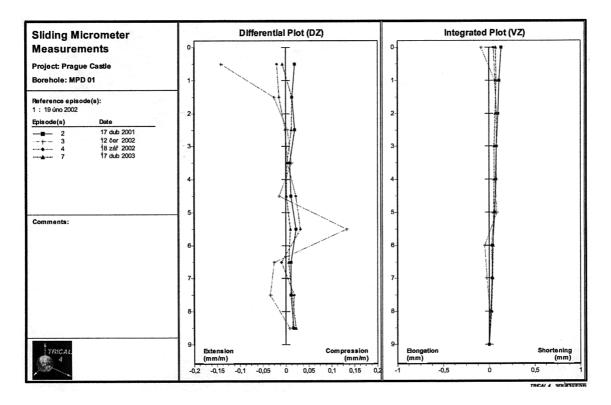
Figure 5: Axial deformation of footing and subsoil: differential and integrated
