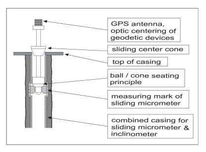
Figure 6: Insert tool to link high accuracy geotechnic and geodetic measurements
