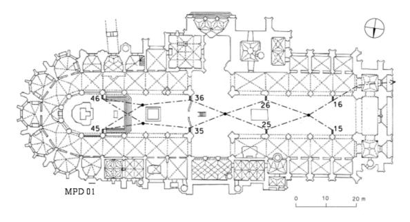
Figure 2: The scheme of benchmarks and locations of sections for trigonometric measurement and MPD 01 reference point at the cathedral
