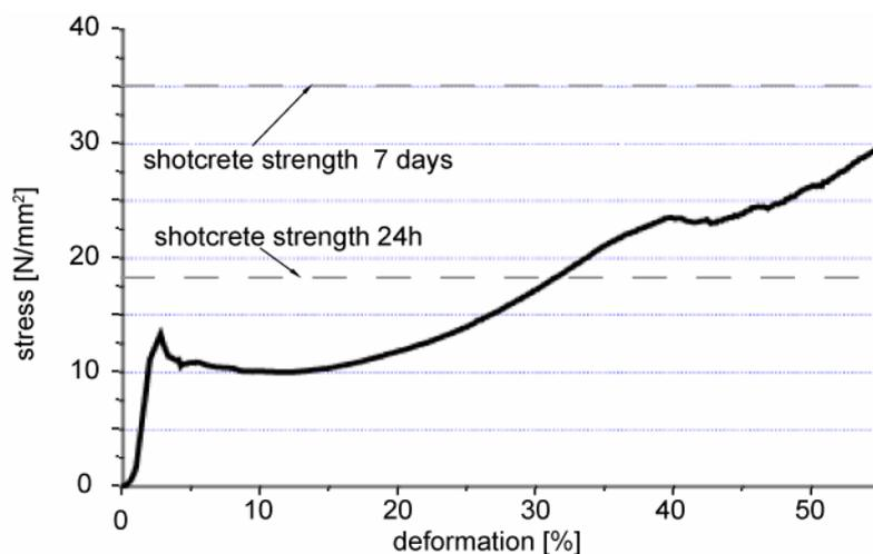
Figure 3: Characteristic Stress – Stain diagram of a HDC element
