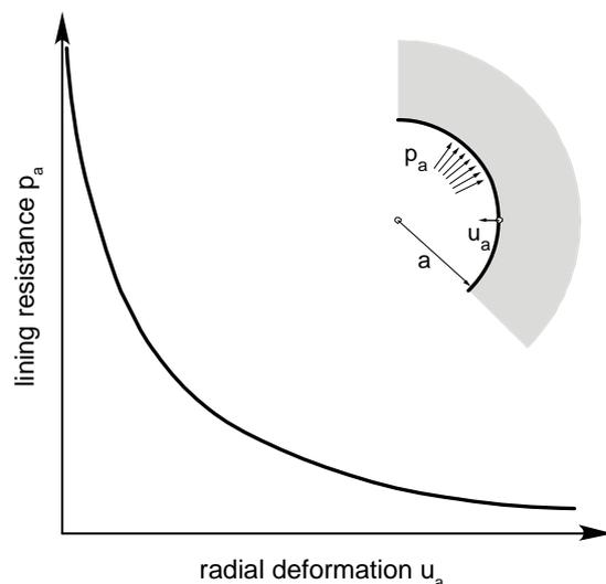
Figure 1: Lining resistance vs. deformation
