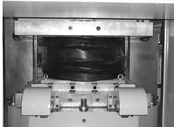
Figure 10: HDC foundation element during load testing
