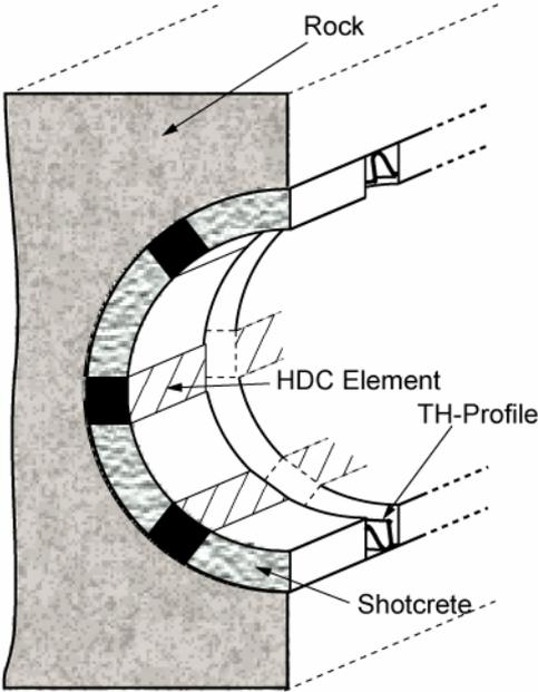
Figure 4 Lining system with HDC Element
