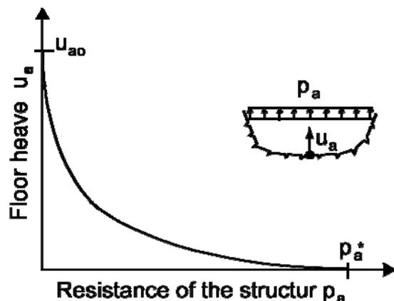
Figure 8: The characteristic line for swelling rock
