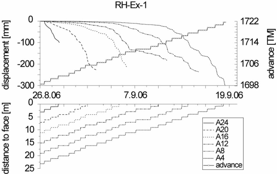
Figure 12 Report of a RH-Extensometer data
