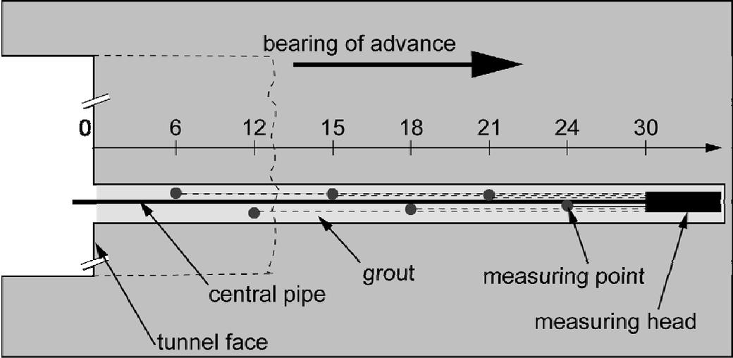
Figure 11: schematic drawing of a RH Extensometer
