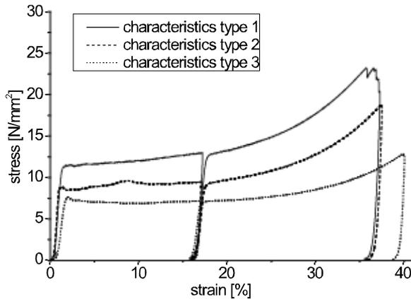
Figure 9: stress – strain – diagram of HDC foundation elements
