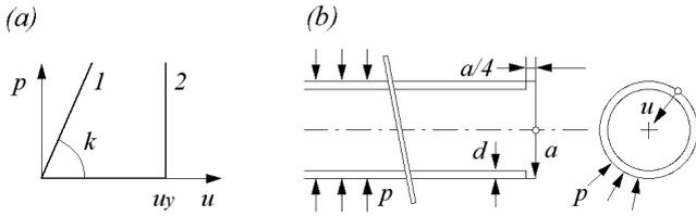
Figure 7. (a) Characteristic lines of support; (b) Problem layout.
