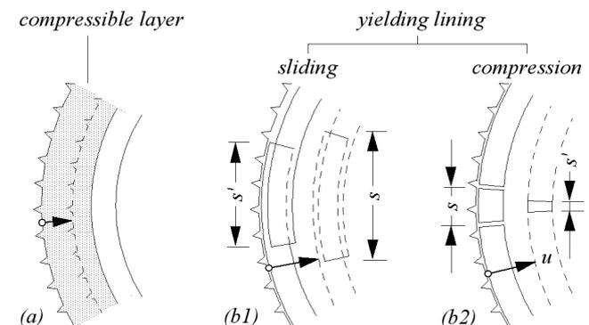
Figure 2. Basic types of flexible support.
