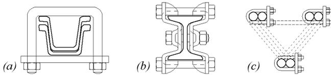
Figure 3. Sliding connections of (a) top hat section steel sets and (b) H section steel sets (from Fröhlich 1948); (c) lattice girders.
