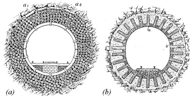
Figure 1. (a) Layer of wood between rock and U section steel sets; (b) Concrete with wood interlayers (from Heise & Herbst 1913).
