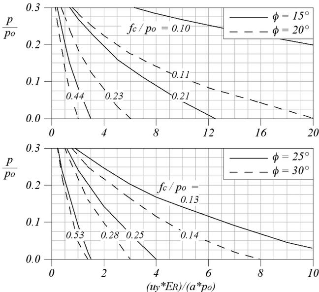
Figure 9. Pressure  $p$  (normalized by the initial stress  $p_0$ ) acting upon a rigid support as a function of the normalized convergence  $u_y$ , occurred during the preceding deformation stage (see Fig. 8 for the other parameters and notation).
