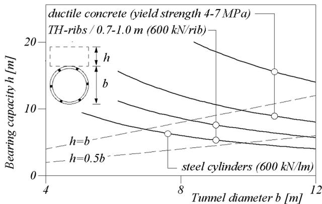
Figure 6. Bearing capacity of yielding support (solid lines) and height of loosening zone (dashed lines) as a function of tunnel diameter  $b$ .
