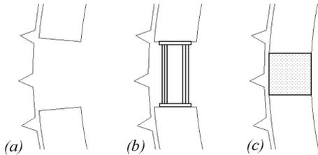
Figure 4. Shotcrete shell with (a) open slots, (b) steel cylinders (Schubert 1996), (c) ductile concrete elements (Thut et al. 2006).
