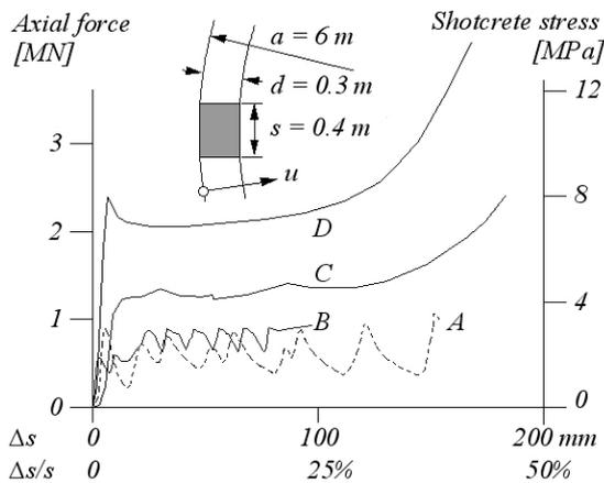
Figure 5. Load-deformation behaviour of compressible elements. Curves A and B: steel cylinders (4 elements per linear meter) after Schubert et al. (1996, 1999), respectively. Curves C and D: ductile concrete elements after Thut et al. (2006).
