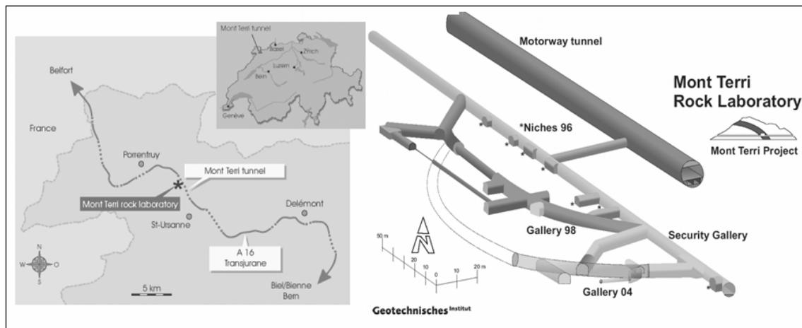
Figure 1: Location map (left) and layout (right) of the Mont Terri Rock Laboratory in NW Switzerland within the Opalinus clay; source: Mont Terri Consortium by Geotechnisches Institut.
