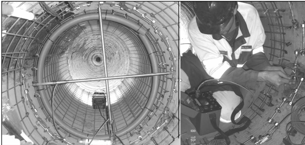
Figure 10: Microtunnel test section with strain gage ring at the tunnel wall and the two surface extensometers (left side), close-up of the strain gage ring and performance of control measurements after the installation (right side); source: Solexperts AG.
