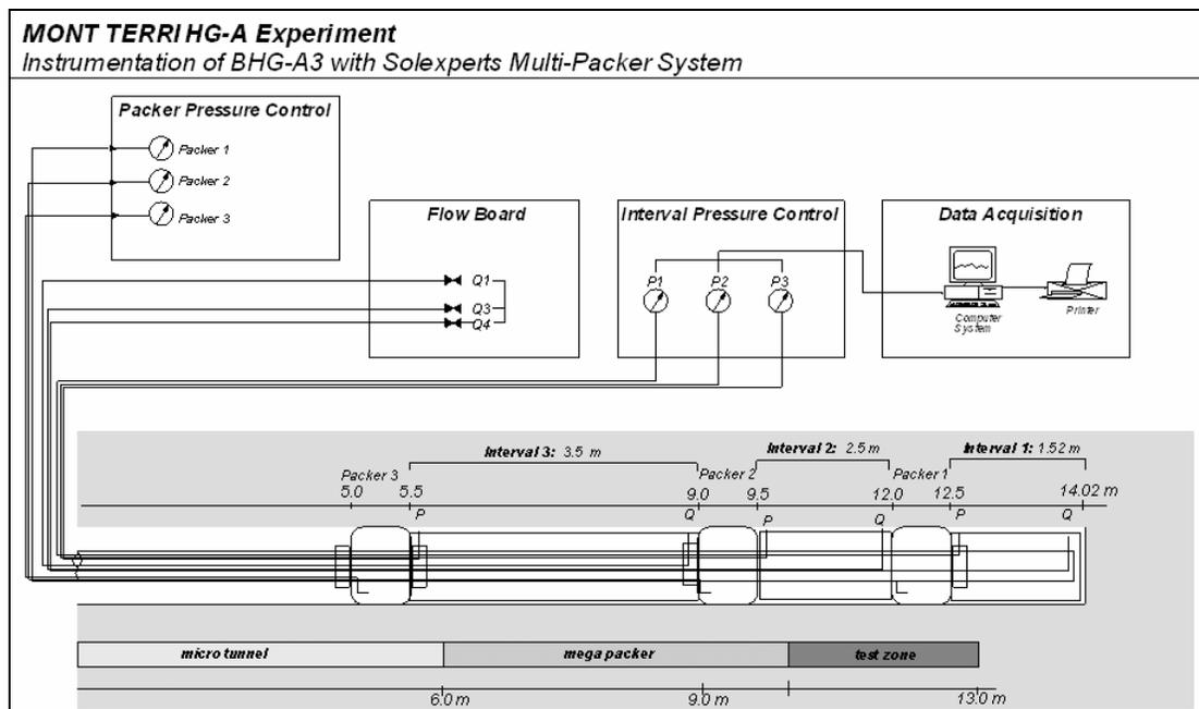
Figure 6: Schematic drawing of the triple packer system installed in borehole BHG-A3 (bottom) and the correspondent surface control units; source: Solexperts AG.
