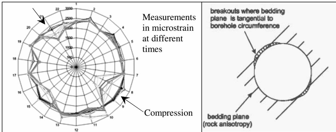
Figure 11: Deformations in the microtunnel measured by the strain gages (left), expected deformations in anisotropic rock (right); source: Mont Terri Consortium.
