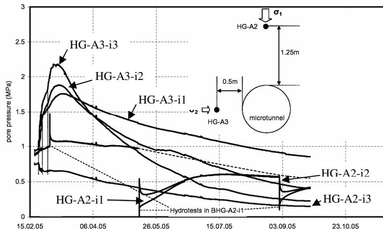
Figure 9: Pore pressure observations during and after the excavation of the microtunnel; source: Mt. Terri Consortium.
