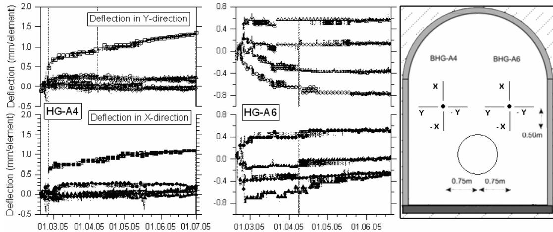
Figure 8: Deflections measured by the chain deflectometers the boreholes BHG-A4 (left) and BHG-A6 (center) and their position relative to the microtunnel (right).
