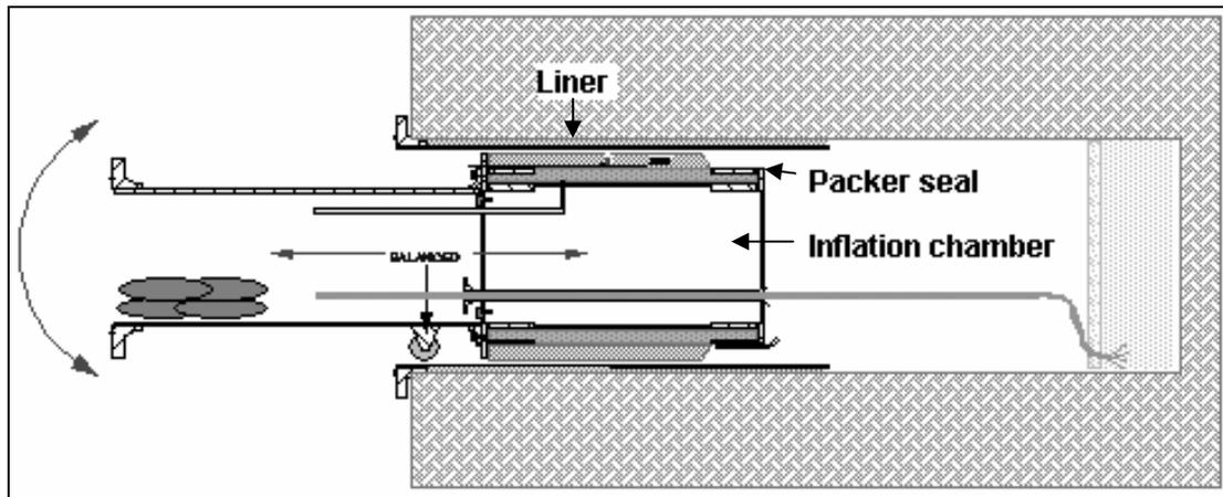
Figure 13: Schematic drawing of the Megapacker emplacement: The Megapacker was rolled through the steel liner and then shifted towards the final position. After leaving the steel liner the Megapacker needed to be balanced. Source: Baski, Inc.
