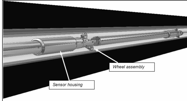
Figure 4: Drawing of the CLINO-chain; source: Solexperts AG.
