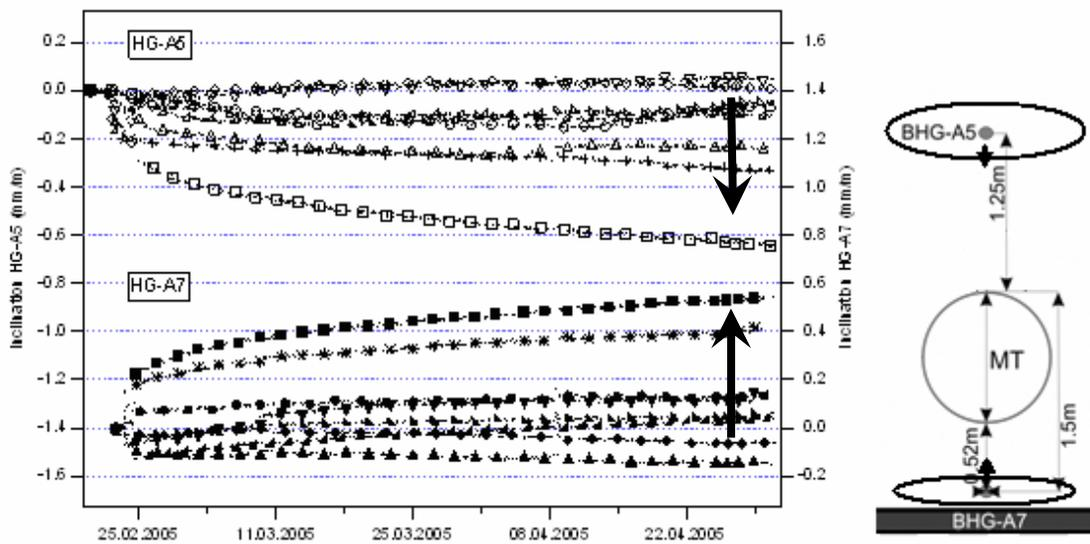
Figure 7: Data plot of the inclinometer chains installed in the boreholes BHG-A5 and BHG-A7 (right side). Location of the axial boreholes BHG-A5 and BHG-A7 in relation to the microtunnel (MT) and the displacement directions (arrows); source: Mont Terri Consortium.
