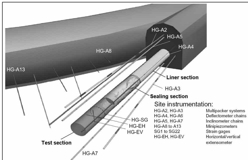
Figure 2: HG-A site with instrumentation of the microtunnel and of the axial boreholes.
