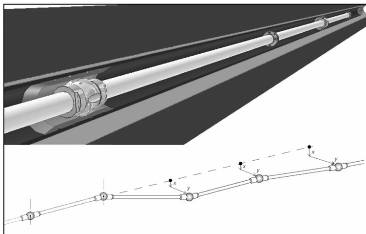
Figure 5: Drawing of the Chain Deflectometer; source: Solexperts AG.
