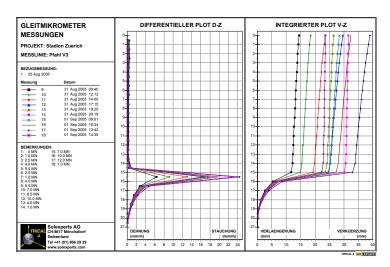
Fig. 3 Sliding Micrometer with cable reel / pile load test stadium Hardturm, strain distribution
