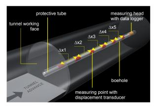
Fig. 8 Reverse Head Extensometer (M-RHX), permanent measurement of displacements during excavation
