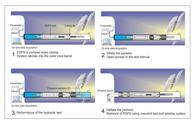
Fig. 7 Pump Down Packer System (PDPS) for hydrogeological testing ahead of the excavation face
