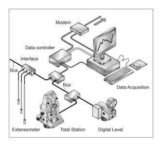
Fig. 11 GeoMonitor 2, automatic data acquisition system
