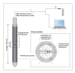
Fig. 2 E-Modulus of rock, Dilatometer probe
