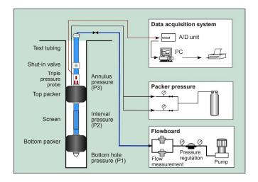
Fig. 5 Hydro testing device
