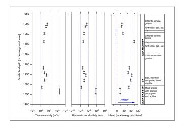
Fig. 6 AlpTransit Lötschberg, Bärsol (Jungfraukeil) profile of hydraulic parameters
