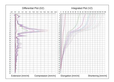
Fig. 4 Instrumented loading test on soft deltaic clays
