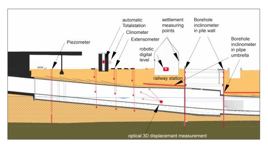
Fig. 10 Basel Luzernerring, schematic view of the tunnel and monitoring
