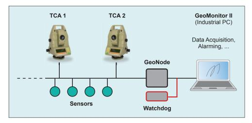
Fig. 14 Automated system GeoMonitor II in the lock chambers of Gabčíkovo waterworks
