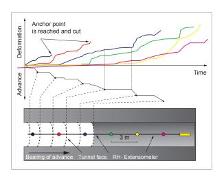
Fig. 9 M-RHX Extensometer measuring results
