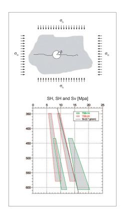
Fig. 1 Stress measurement, Hydro Frac tests
