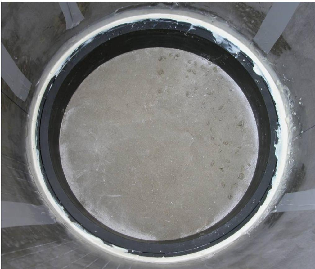
**Fig. 5:** Solexperts TDR ring sensor after emplacement: The gap between sensor and reservoir wall is filled with resin to prevent gas and water flow
