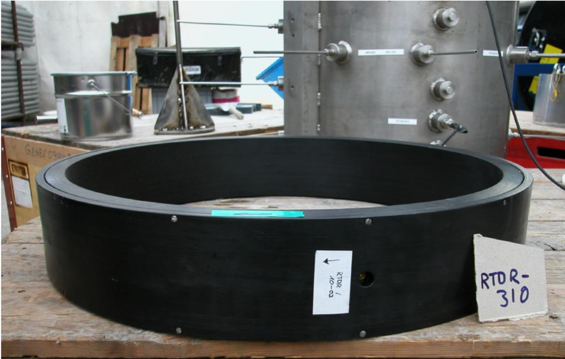
**Fig. 4:** Solexperts TDR ring sensor before emplacement
