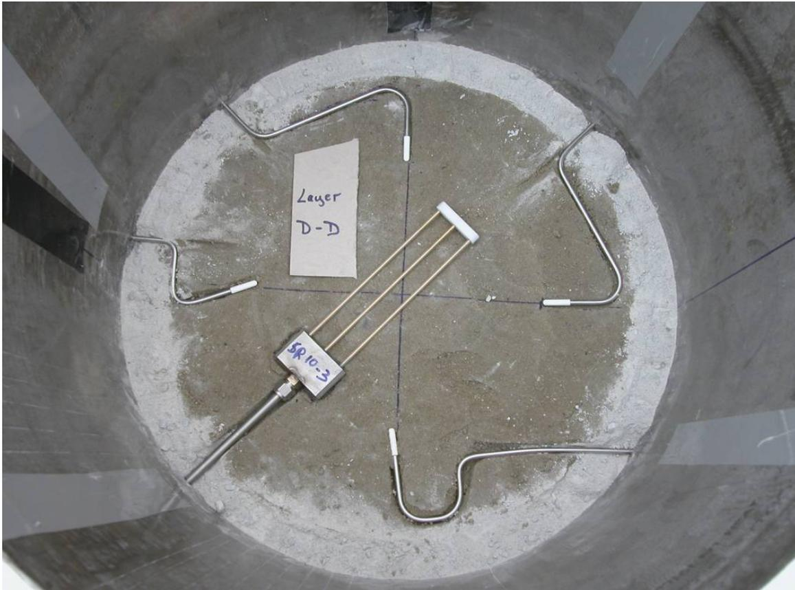
**Fig. 3:** Solexperts TDR high pressure rod sensor (and tensiometers) during installation for an experiment
