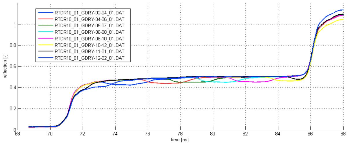
**Fig. 6:** TDR signals measuring spatially changing dielectric permittivity along the ring sensor
