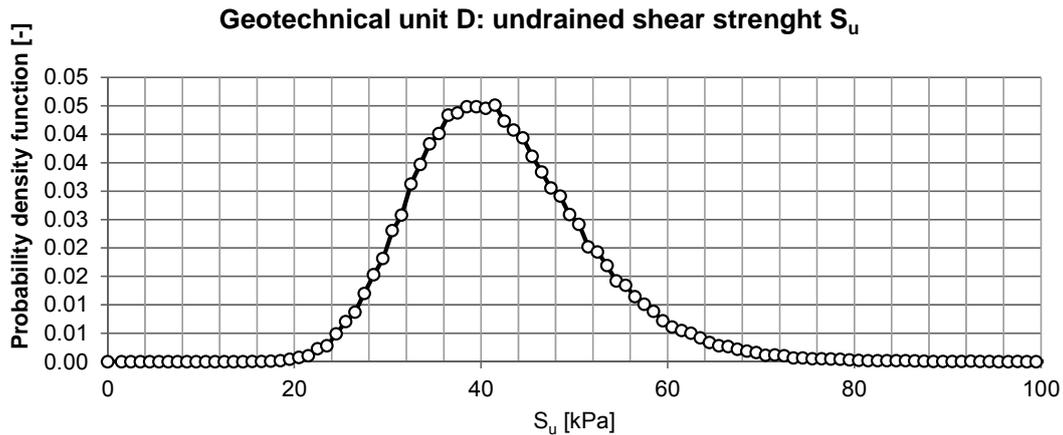
**Figure 5** Probability density function of the undrained shear strength  $S_u$  for geotechnical Unit D
