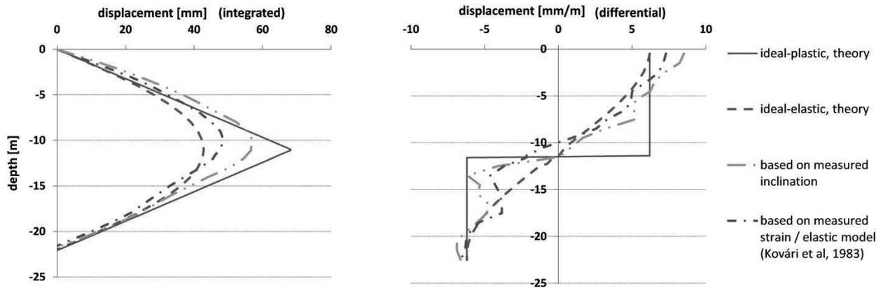
**Figure 15** Wall displacements in theory and as measured (after final excavation, head displacement set to zero). TRIVEC measurements show the yielding of the retaining wall
