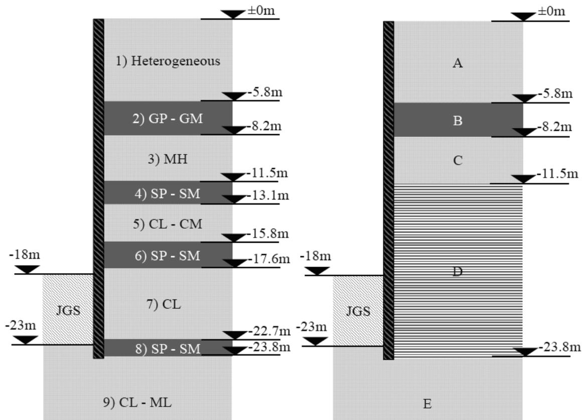
**Figure 4 Comparison between soil layers and geotechnical units**
