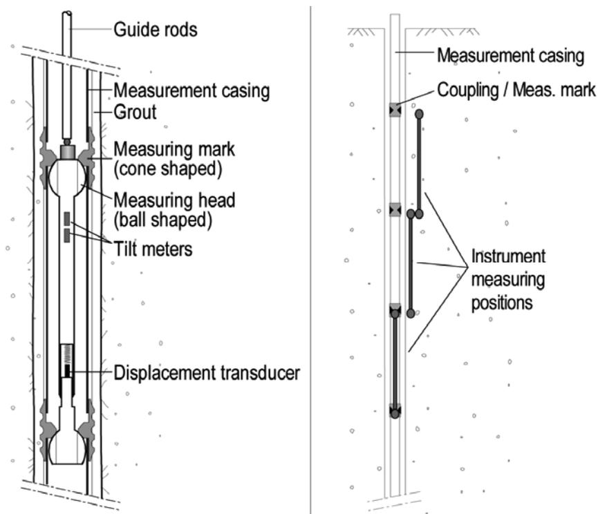
**Figure 7** (a) TRIVEC instrument in measuring tube; (b) stepwise placing of the TRIVEC in the measurement tube
