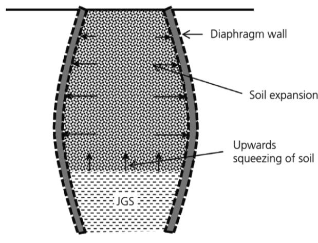
**Figure 13** Expansion of the volume inside the shaft due to the insertion of the jet grout columns (after Rabaiotti et al. 2015)
