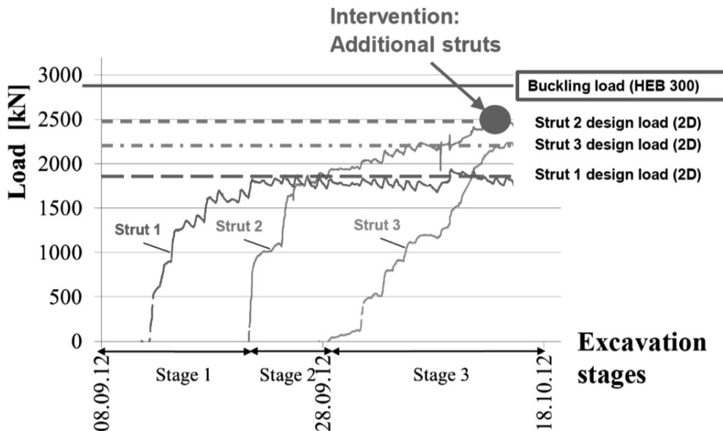
Figure 12 Measured and design forces of the struts during excavation
