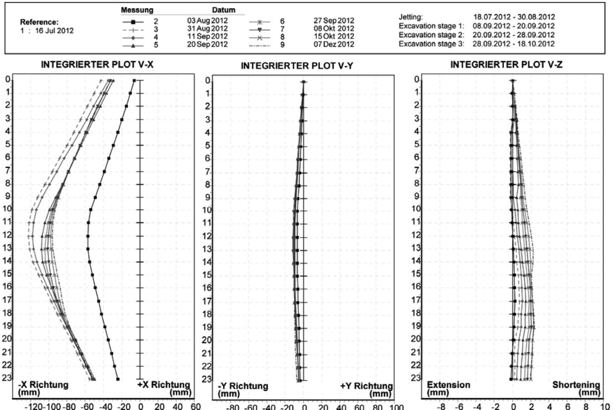
**Figure 8** Integrated TRIVEC Measurements in the retaining wall (outer side); (a) horizontal displacements rectangular to the wall; (b) horizontal displacements in wall direction; (c) cumulated strain
