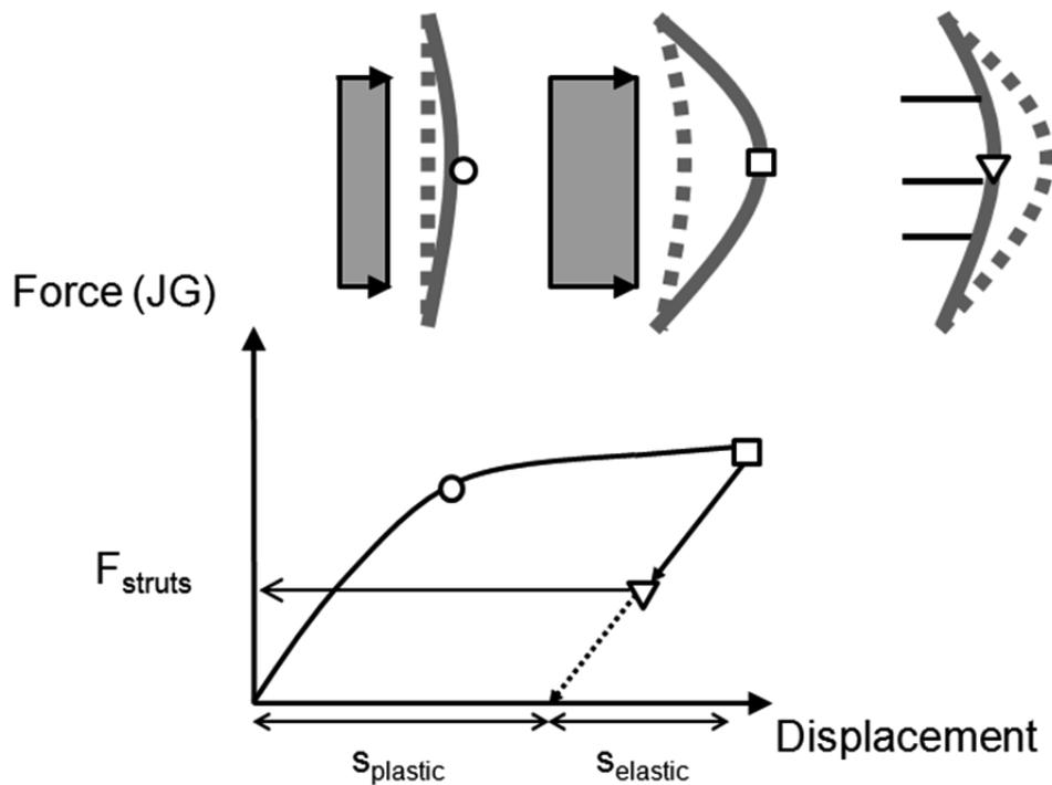
**Figure 16** Mechanism illustrating the deformation, elastic rebound of the struts and increased forces in the struts, in addition to those due to earth pressure. The grey beam shows the wall, the grey rectangle the pressure induced by the jet grouting and volume increase inside the shaft
