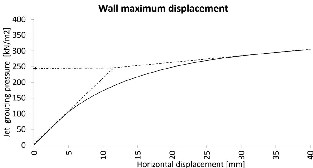
**Figure 14** Yielding of the retaining wall starts at jetting pressures exceeding 200 to 250 kN/m<sup>2</sup>
