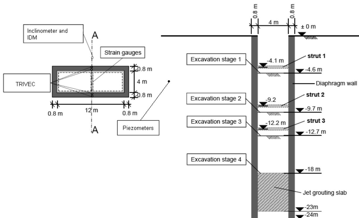
**Figure 6** Plan view and cross-section of the test shaft indicating the depth of the struts and excavation stages as well as the installed instrumentation
