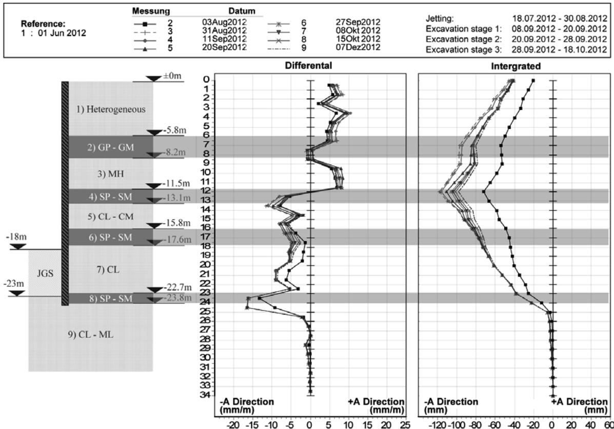
**Figure 9** Inclinometers measurements 1.5 m beside the shaft show displacements in similar order of magnitude. Differential displacements correspond with the soil stiffness
