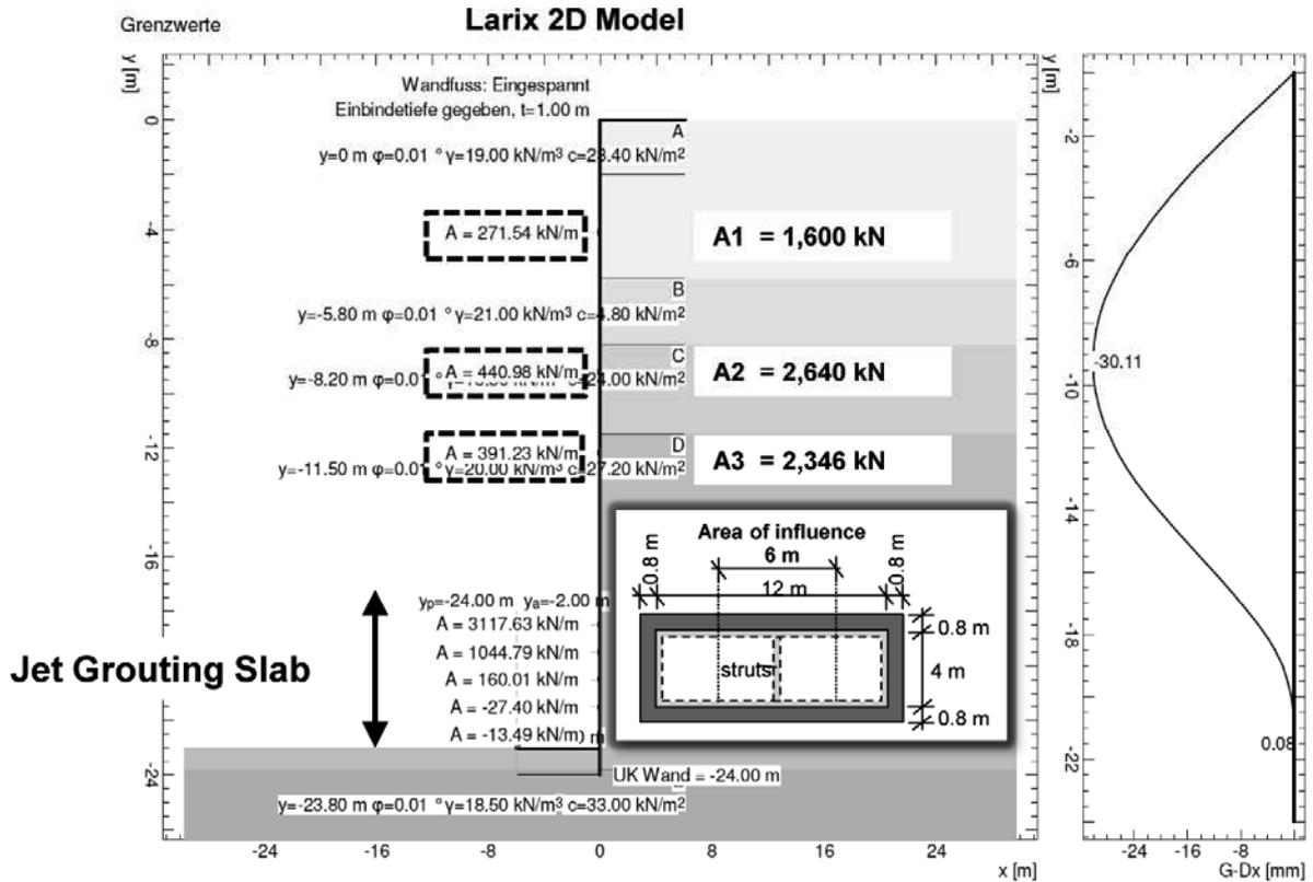
Figure 11 Design strut forces as determined by truss analysis
