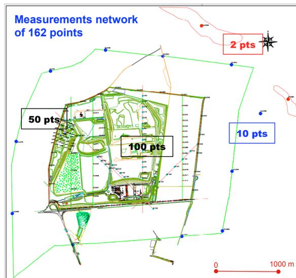
Figure 1: Experimental network (162 points) for gas measurements on Claye-Souilly site.
