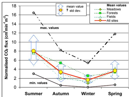
Figure 4: Evolution of the average fluxes in France according to the type of ground and the season. Measurements by INERIS accumulation chamber on the 2007-2009 period.
