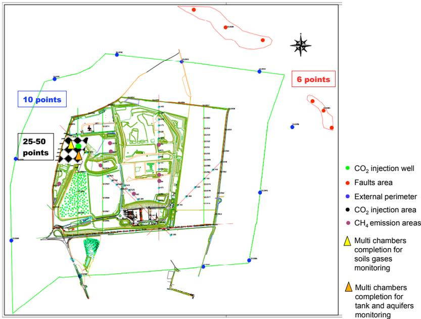
Figure 5: First matrix of location of the reference measurement points for a geochemical survey of Claye Souilly site.
