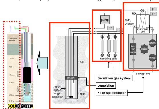
Figure 6: Technical details of the platform for continuous geochemical monitoring of gases that should be implemented on the Claye Souilly site.
