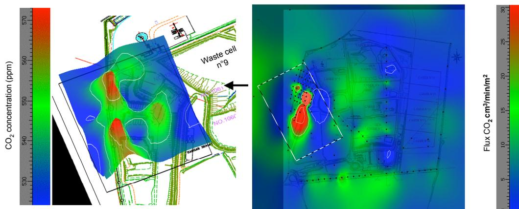
Figure 2: Typical 2D/3D interpolated map of CO<sub>2</sub> surface monitoring (October 2010):
