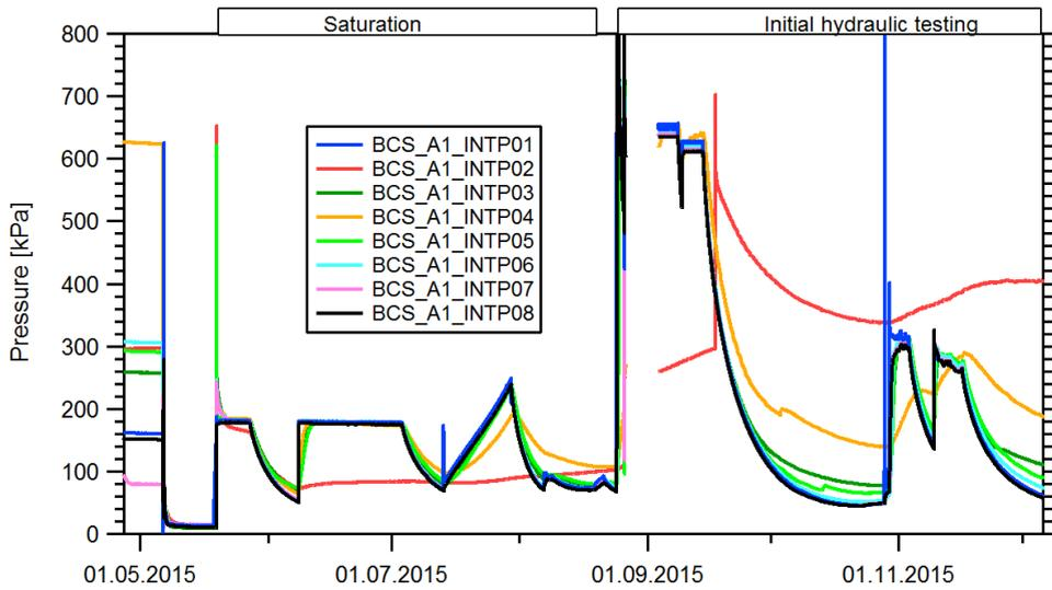
Figure 6. Re-saturation of CS-A experiment mock completion installation after air drilling.
