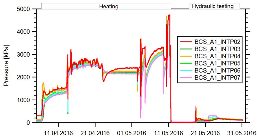
Figure 9. Mock completion pressure test response in the cased and cemented hole section during the heating-cooling cycle.
