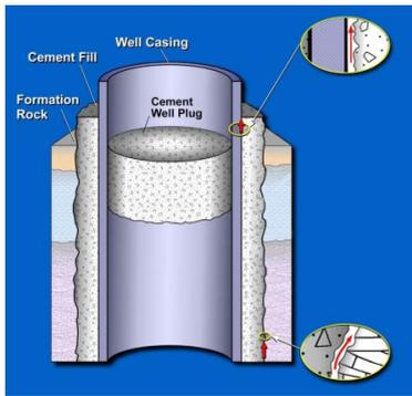
Figure 2: Well system leakage mechanisms at casing / cement and cement / rock formation boundaries (modified after IPCC 2005 report [1]).
