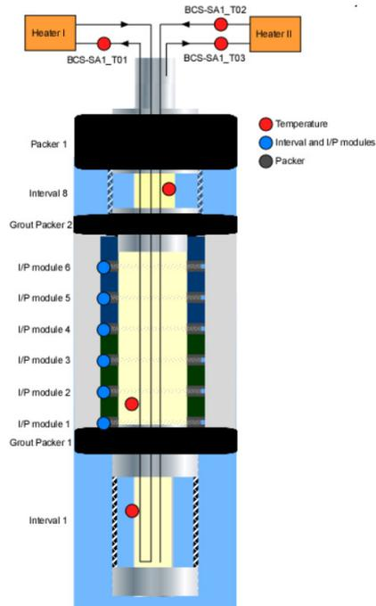
Figure 5. Mock completion injection / extraction access design for the CS-A experiment.
