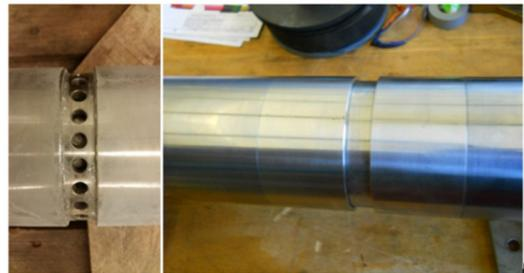
Figure 4. (a) Casing with 6 I/P modules and grout packers, (b) left: I/P module with open valve; right: I/P module valve closed.
