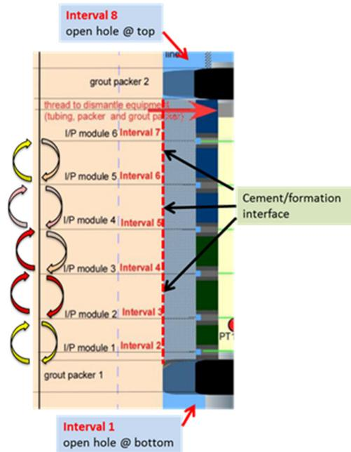
Figure 11. CS-A experiment flow interpretation along the outer cement sheath/formation boundary.
