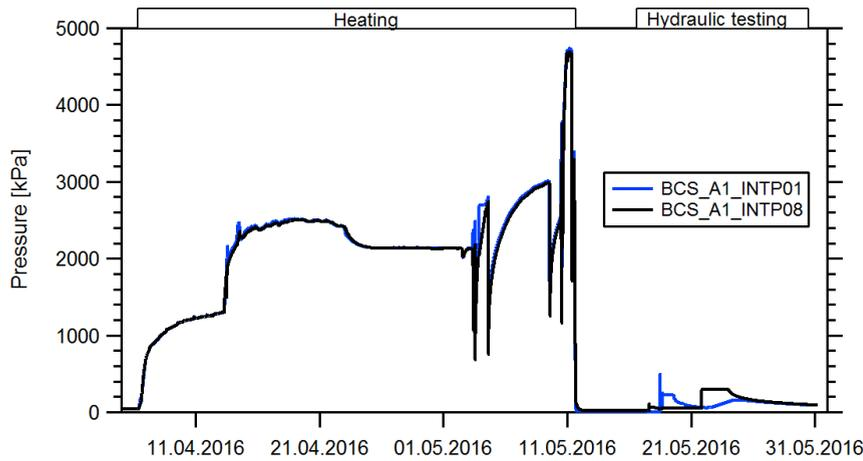
Figure 10. Mock completion pressure test response in the open hole chamber intervals 1 and 8 during the heating-cooling cycle.
