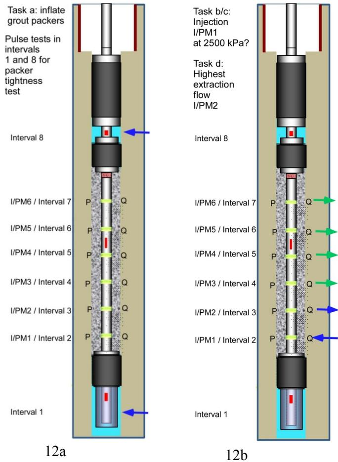
Figure 12. Mock completion injection / extraction access design.
