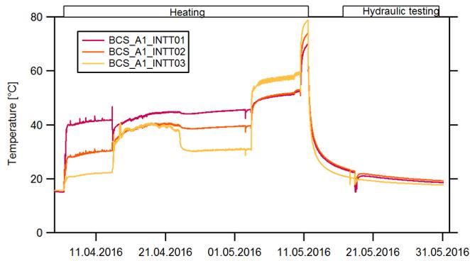
Figure 8. Mock completion heat/cool cycling 06 April 2016 to 01 June 2016 for micro-annuli creation.
