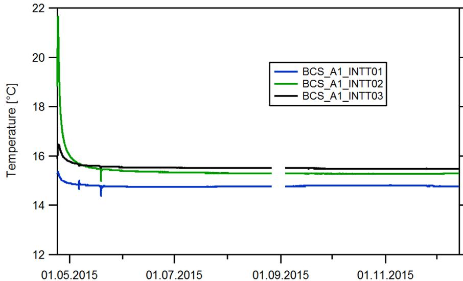
Figure 7. Temperature profile after CS-A equipment installation. Temperature sensors placed in lower open hole chamber interval 1 (BCS\_A1\_INTT01), in the cased and cemented section (BCS\_A1\_INTT02) and in the upper open hole chamber interval 8 (BCS\_A1\_INTT03).
