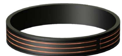
Ring shape TDR sensor for barrier experiment (schematic)
