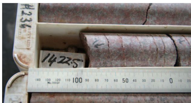
Fig. 3 Example of saddle-shaped discing/fragmentation near 1,422.5 m depth (after Bungler 2010)
