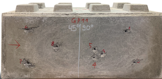
baLCon element type A, test according to VPAM; GP11 (7.5 x 55) 90° & 45°
