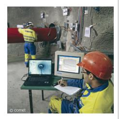
The Solexperts GeoMonitor System provides a practical solution for automatically monitoring many instruments and sensors and handling large amounts of measurement data from complex sites.
