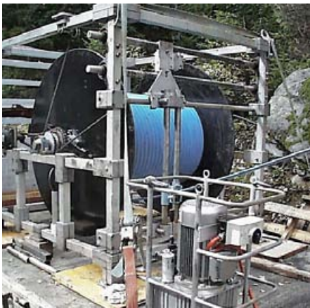
Winch with measuring cable and hydraulic power unit on transport vehicle
