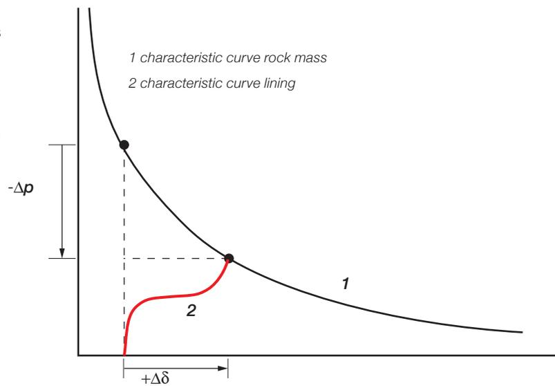
In heavily squeezing rock conditions the installation of large I-sections with a high deformation capacity is more efficient. hiDSte elements in combination with I-sections offer the desired high deformability in combination with high lining resistance. The load-deformation mechanism is illustrated by the adjacent figure. It shows the characteristic line of the rock mass and that of the deformable lining. Allowing a convergence  $\Delta u$  reduces the ground pressure by  $\Delta p$ .
