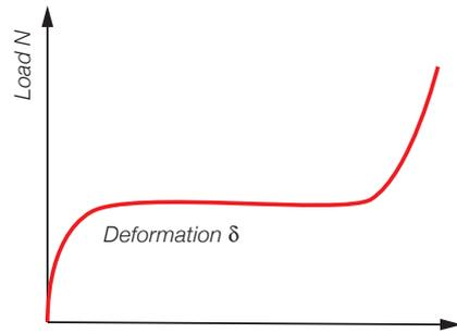
The hiDSte element is basically a thick-walled cylinder which deforms plastically. After an initial elastic deformation the stress- strain curve exhibits a large deformation capacity at a high load level. The properties of the element are based on the size of the I-section, the number of elements per arch and the required convergence.
