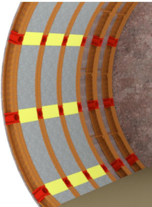
The combination of hiDCon and hiDSte elements in a lining is shown schematically in the picture above. It is possible to install the steel arches first directly at the tunnel face. The shotcrete support with the hiDCon elements is then installed later at a certain distance.
