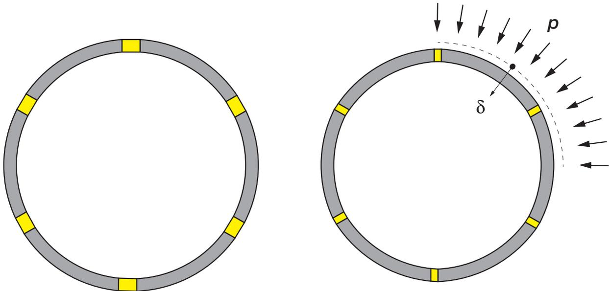
When tunnelling in squeezing ground large deformations (convergence) or high rock pressure may arise. To overcome such zones the most economical solution consists in applying a deformable lining system avoiding re-profiling and reconstruction of the tunnel. It has the advantage of being safe and time efficient. A number of deformable elements are placed in the shotcrete lining between TH-steel profiles or lattice girders.
