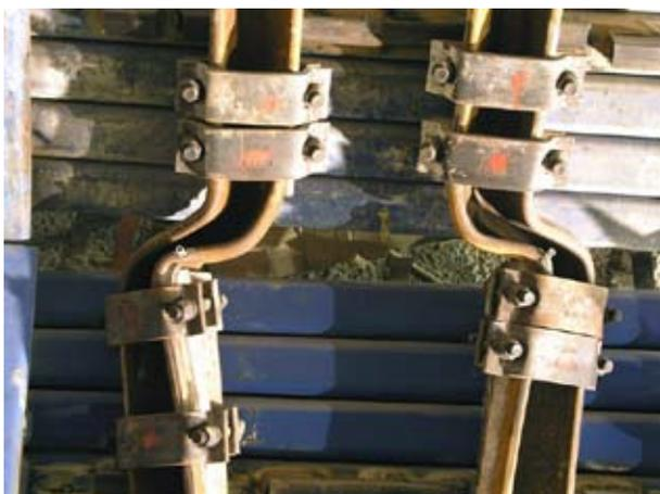
Fig. 7: Steel arches loaded up to local buckling of the ribs (TH44)
