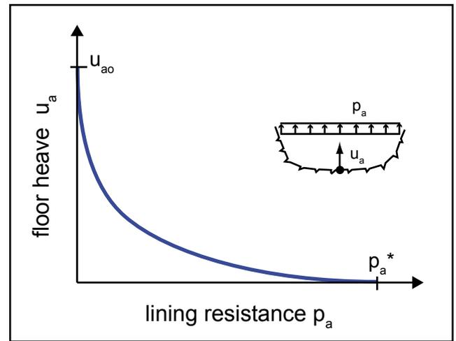
Fig. 17: Characteristic line of swelling rock
