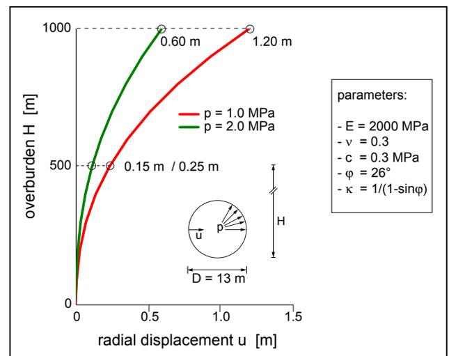
Fig. 13: Radial displacement  $u$  versus height of overburden  $H$  for two values of lining resistance  $p$  (Kovári and Ehrbar, 2008)
