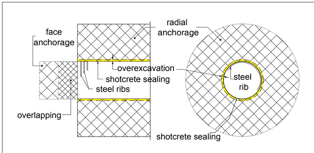
Fig. 14: Schematic representation of the excavation-support concept (Kovári and Ehrbar, 2008)
