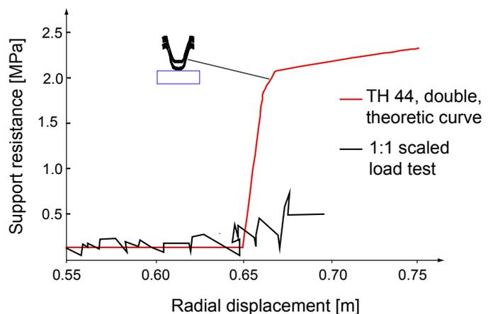
Fig. 8: Test results and theoretically expected diagrams for single and double ribs
