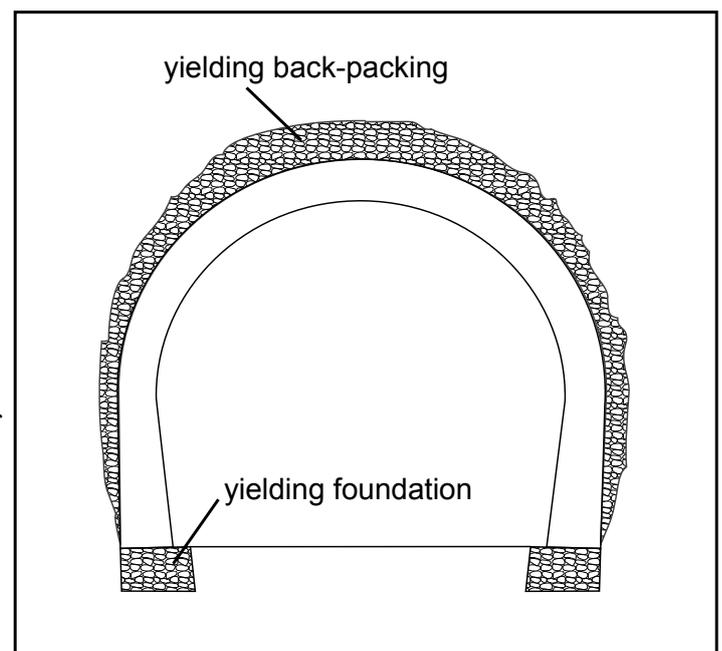
Fig. 4: Tunnel lining in swelling rock: yielding back-packing in the roof and yielding foundation (Schächterle, 1926)
