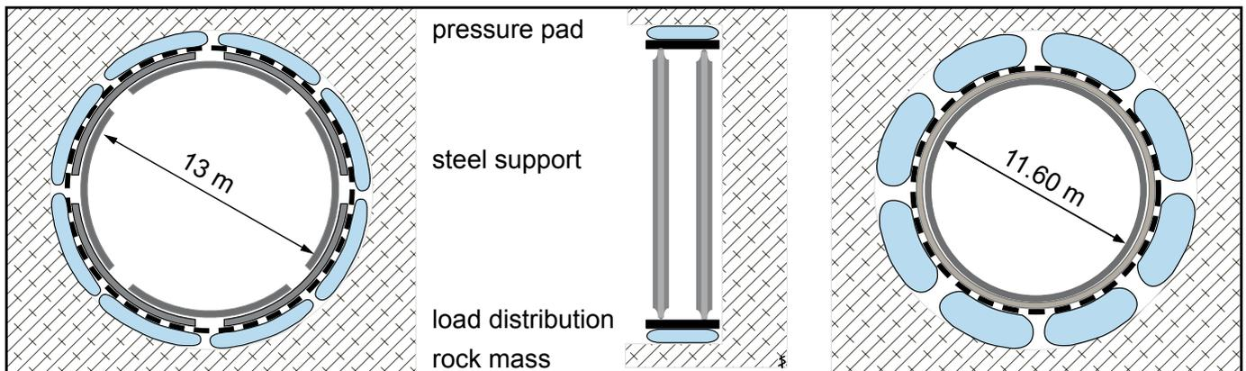
Fig. 6: Field test of a large diameter steel support executed in a hard rock niche with two complete steel sets, (a) The sets prior to loading, (b) The sets after loading by water-inflatable cushions and convergence up to 0.7 m (Kovári et al, 2005)
