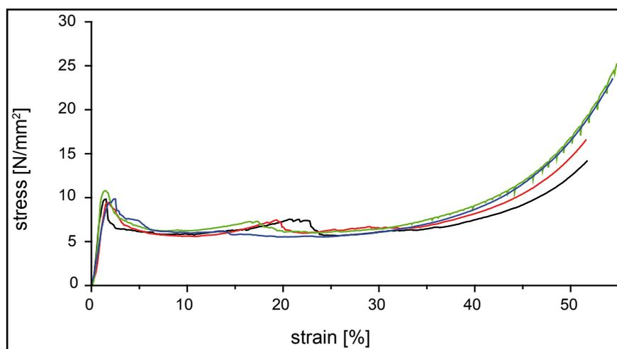
Fig. 11: Stress-strain behaviour of yielding concrete elements
