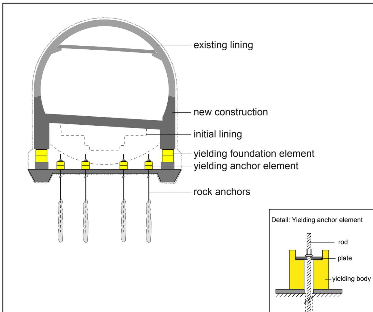
Fig. 16: Chienberg Road Tunnel in heavily swelling rock: “Modular Yielding Support”
