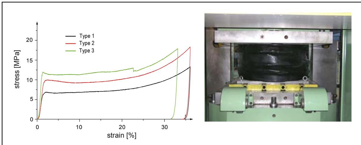
Fig.18: Laboratory tests of cylindrical foundation elements (height: 1000 mm / diameter 900mm)
