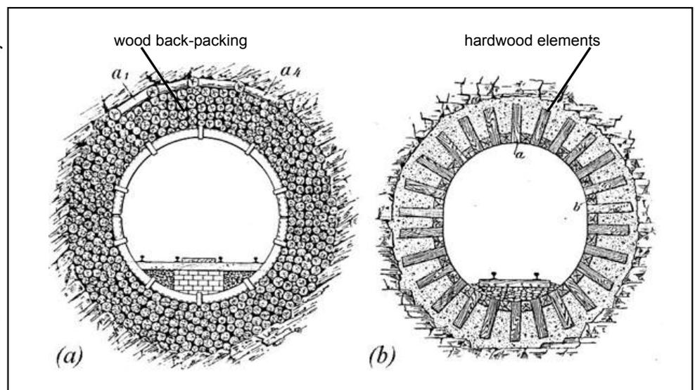
Fig. 1: Yielding support concepts. (a) Back-packing with wood between steel support and rock, (b) Interlayer of wooden panels in the concrete lining (Heise and Herbst, 1913)
