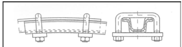
Fig. 3: Sliding steel rib connection (Fröhlich, 1948)
