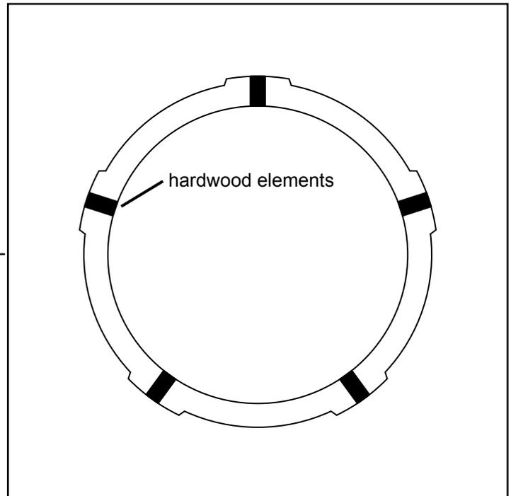
Fig. 2: Yielding hardwood elements between prefabricated concrete segments (Lenk, 1931)
