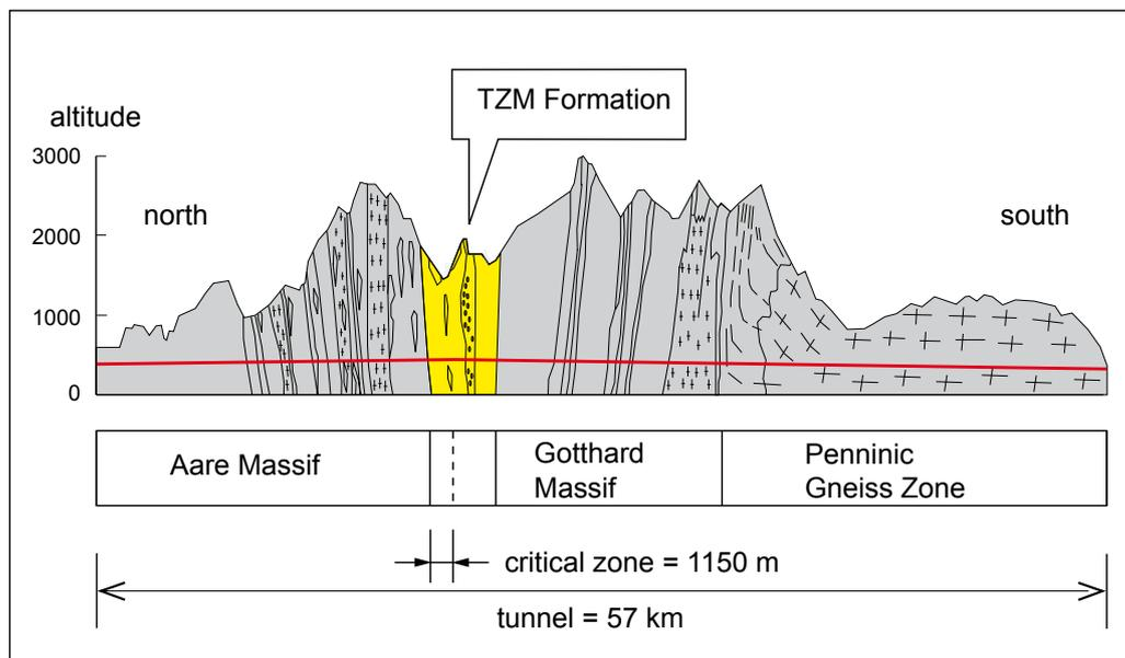
Fig. 12: Gotthard Base Tunnel: schematic representation of the longitudinal geological section with the squeezing TZM-Formation
