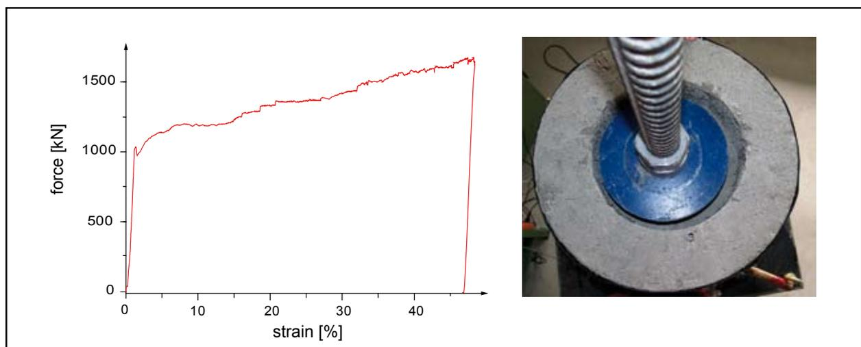
Fig.19: Laboratory test of a cylindrical anchor element
